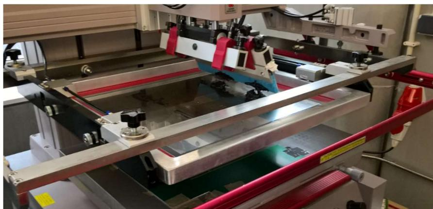
**Figure S1.** Stencil printing equipment used to deposit electrically conductive composites on the PCB's.
