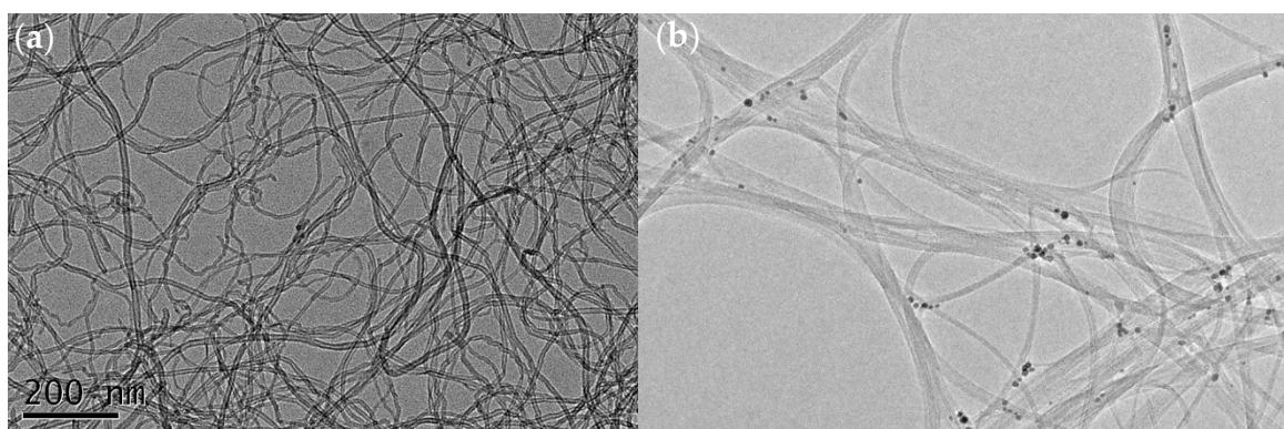
**Figure S2.** Transmission electron microscopy images of (a) individual MWCNTs NC7000 and (b) ropes of SWCNTs Tuball (obtained from OCSiAl site: <https://ocsial.com/en/material-solutions/tuball/>).
