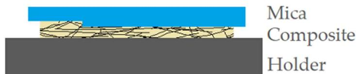
**Figure S4.** Schematic of the preparation of the samples for AFM analyze, with depiction, left side of the mica lamella, of the reason for the appearance off the atomic terrace observed in Figure 7a.
