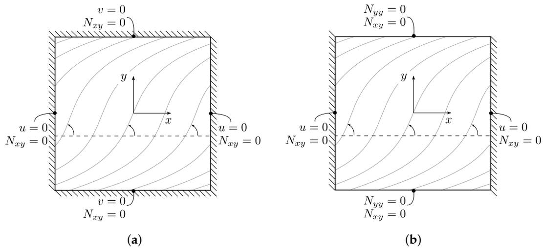
**Figure 3.** Pre-buckling boundary conditions for fiber variation along  $y$ : (a) Case-Ty1; (b) Case-Ty2.
