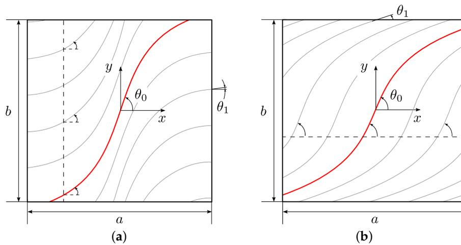
**Figure 1.** Panel geometry and reference system: (a) fiber variation along the  $x$ -direction; (b) fiber variation along the  $y$ -direction.
