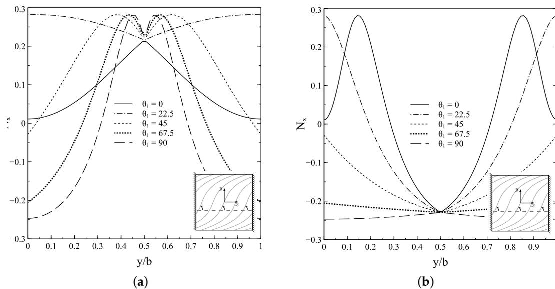
**Figure 7.** Pre-buckling membrane resultants for  $[\pm \langle \theta_0 | \theta_1 \rangle_y]_s$  laminates subjected to Case-Ty2 conditions: (a)  $\theta_0 = 15$ ; (b)  $\theta_0 = 75$ .
