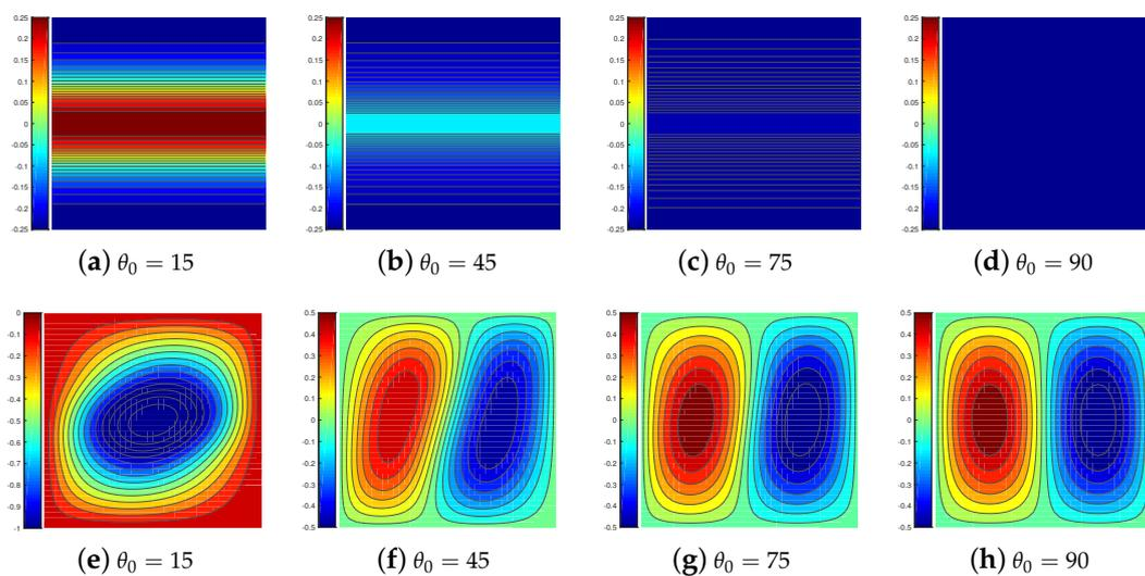
**Figure 9.** Pre-buckling and buckling results for SSSS variable-stiffness configurations,  $b/h = 50$ , and  $[\pm < \theta_0 | 90 >_y]_s$ : (a)–(d): pre-buckling distribution of internal forces  $N_{xx}$ , (e)–(h): buckling mode.
