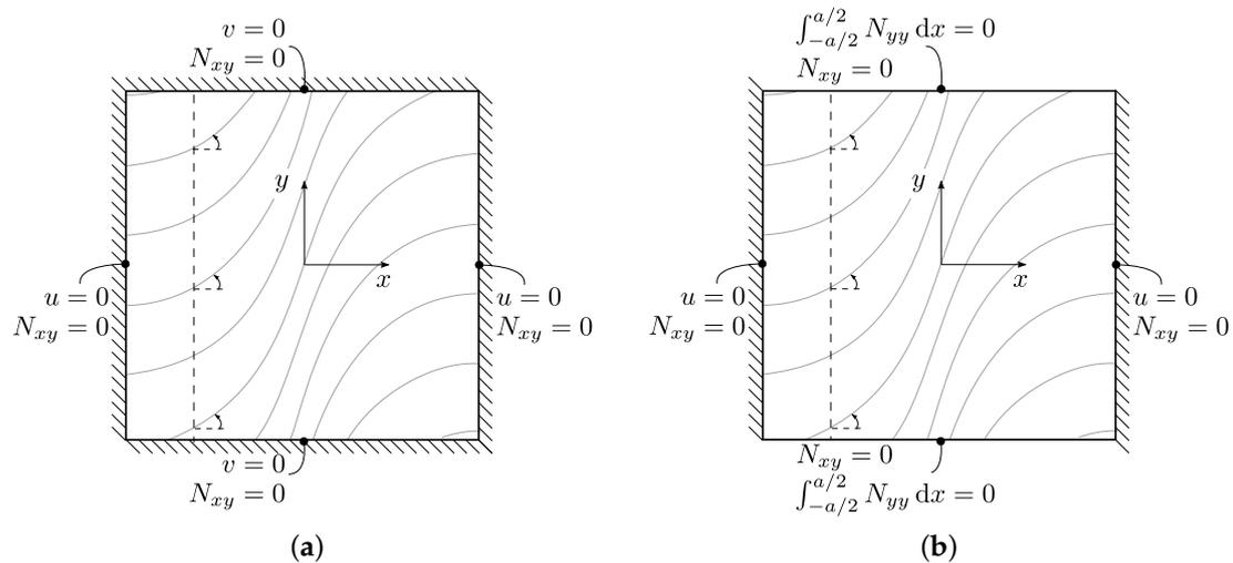
**Figure 2.** Pre-buckling boundary conditions for fiber variation along  $x$ : (a) Case-Tx1; (b) Case-Tx2.
