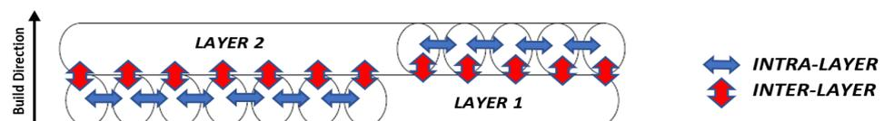
**Figure 11.** Interlayer and intralayer bonds formed between deposited roads. Reconstructed based on Gurralla et al. [76].
