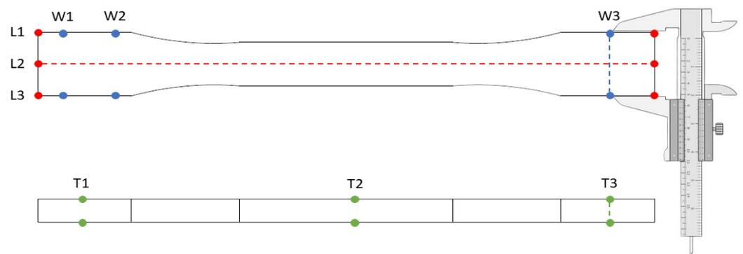
**Figure 2.** Different locations of measurement for the width (blue marking), length (red marking), and thickness (green marking); dotted lines indicate measured ends.
