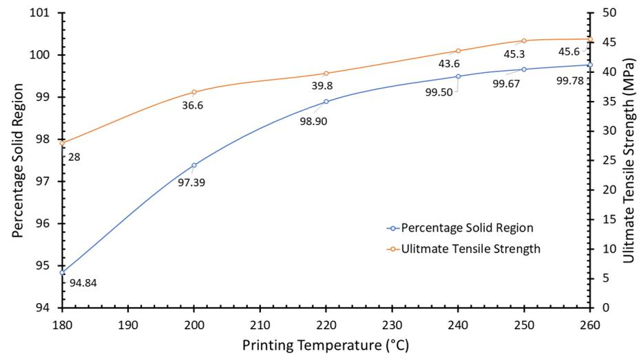
Figure 9. Ultimate tensile strength and percentage of solid region against printing temperature.
