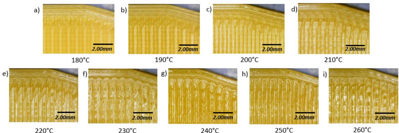
**Figure 5.** Physical appearance of specimens printed at different printing temperatures: (a)  $T = 180\text{ }^{\circ}\text{C}$ , (b)  $T = 190\text{ }^{\circ}\text{C}$ , (c)  $T = 200\text{ }^{\circ}\text{C}$ , (d)  $T = 210\text{ }^{\circ}\text{C}$ , (e)  $T = 220\text{ }^{\circ}\text{C}$ , (f)  $T = 230\text{ }^{\circ}\text{C}$ , (g)  $T = 240\text{ }^{\circ}\text{C}$ , (h)  $T = 250\text{ }^{\circ}\text{C}$ , and (i)  $T = 260\text{ }^{\circ}\text{C}$ .
