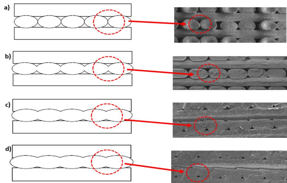
**Figure 12.** Schematic of the reconstructed bond development and SEM images at 50 $\times$  magnification detailing the fracture surface of tensile testing specimens printed at: (a)  $T = 180\text{ }^{\circ}\text{C}$ , (b)  $T = 200\text{ }^{\circ}\text{C}$ , (c)  $T = 240\text{ }^{\circ}\text{C}$ , and (d)  $T = 260\text{ }^{\circ}\text{C}$ .
