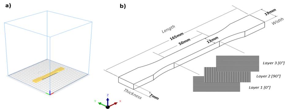
**Figure 1.** (a) Print orientation and (b) dimensions of the specimen according to the ASTM D638-14 Type 1 Standard [66].
