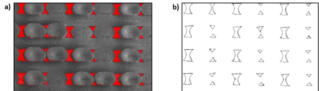
**Figure 4.** (a) Adjustment of threshold to determine the average size and percentage of void. (b) Binarized form of micrograph.
