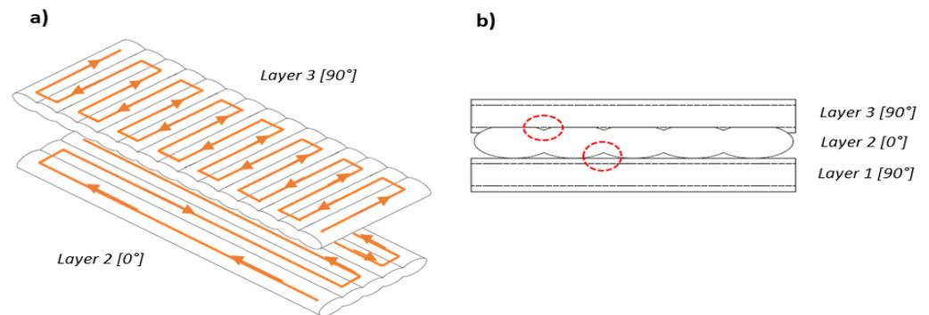
**Figure 13.** (a) Printing path (orange) during the fabrication of specimens. (b) Overlap of deposited roads with the previous layer (circled in red).
