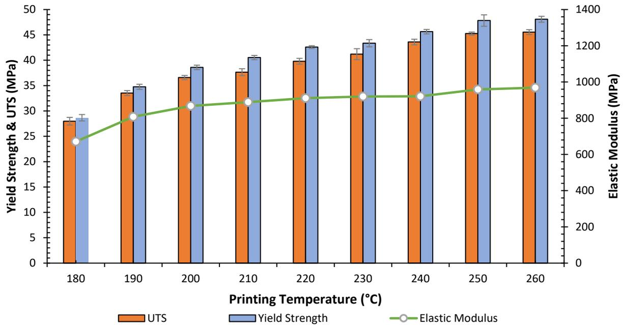
Figure 6. Ultimate tensile strength (UTS), yield strength, and elastic modulus at different printing temperatures.
