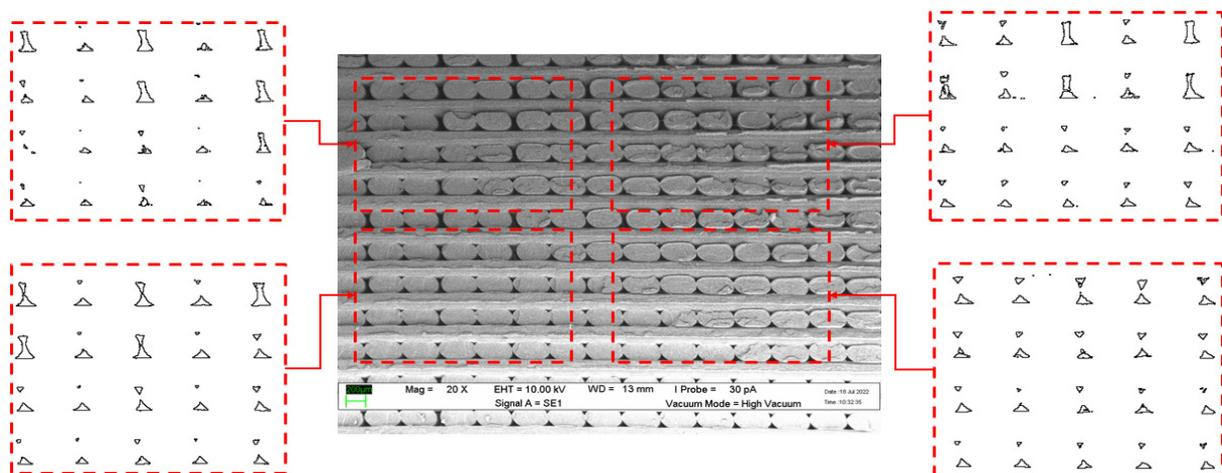
Figure 3. Example of selected regions used to conduct analysis to determine the formation of voids.
