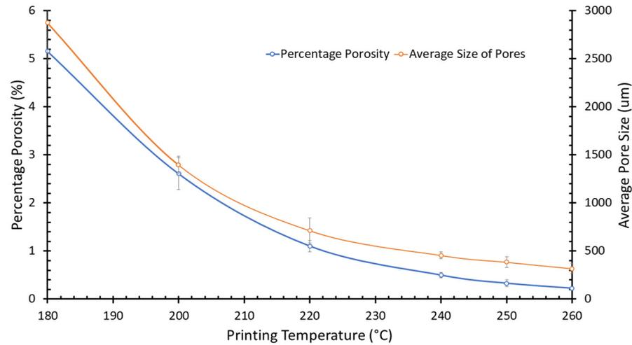
Figure 8. Percentage area of voids and average void size plotted against printing temperature.
