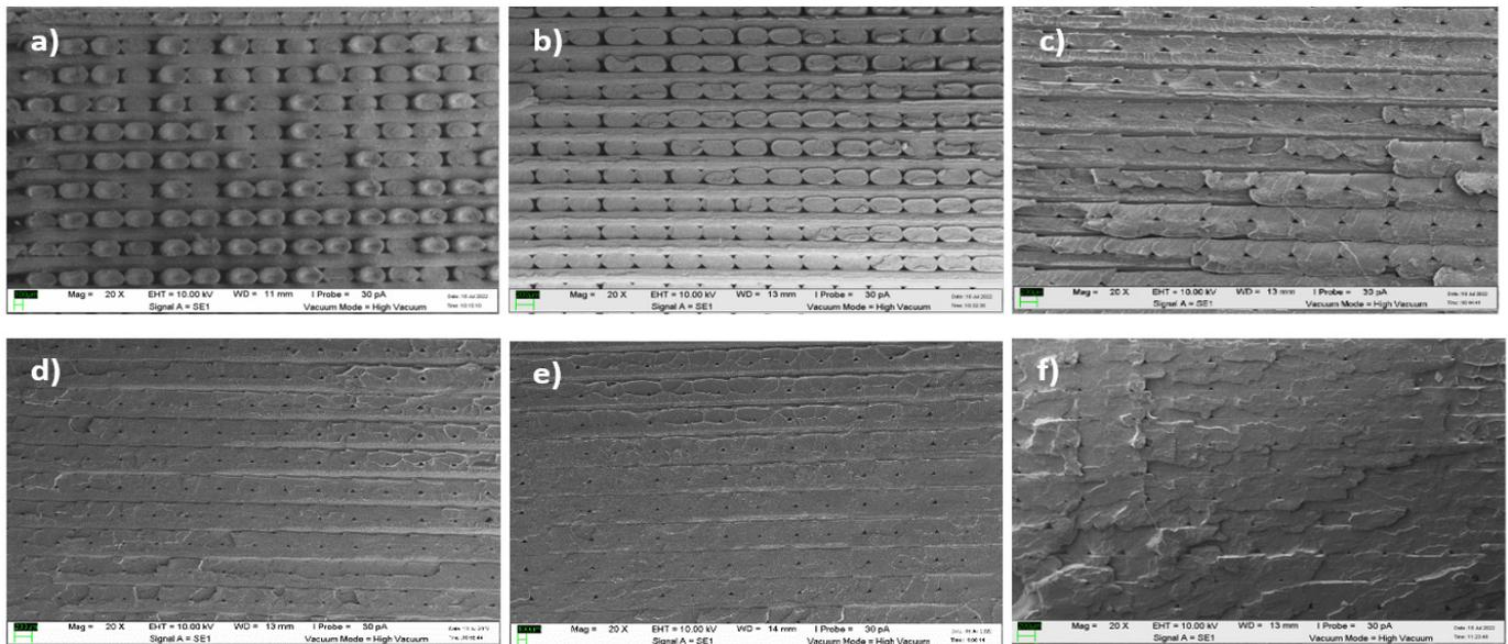
**Figure 10.** SEM images at  $20\times$  magnification detailing the fracture surface of the tensile testing specimens printed at: (a)  $T = 180^\circ\text{C}$ , (b)  $T = 200^\circ\text{C}$ , (c)  $T = 220^\circ\text{C}$ , (d)  $T = 240^\circ\text{C}$ , (e)  $T = 250^\circ\text{C}$ , and (f)  $T = 260^\circ\text{C}$ .
