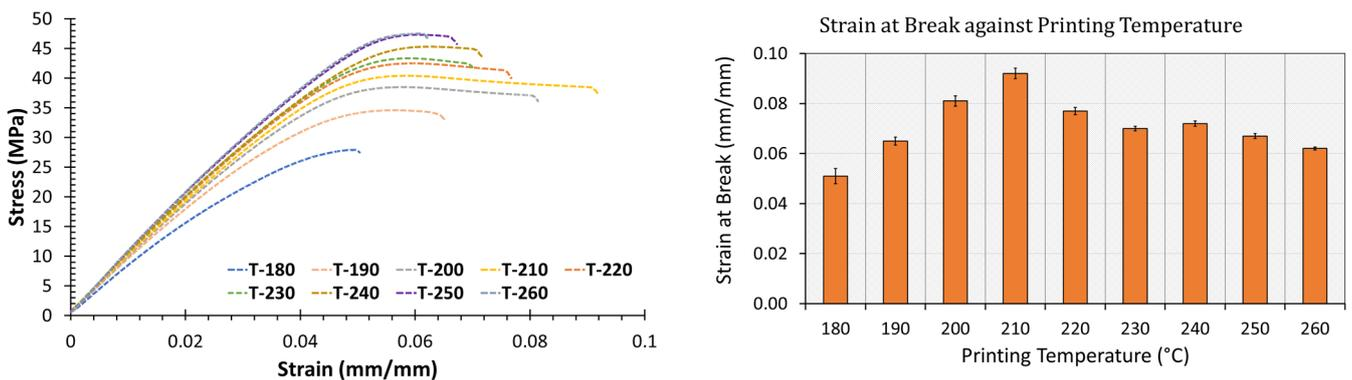
Figure 7. Stress–strain curve at different printing temperatures; values at the end of each curve represent the strain at break.
