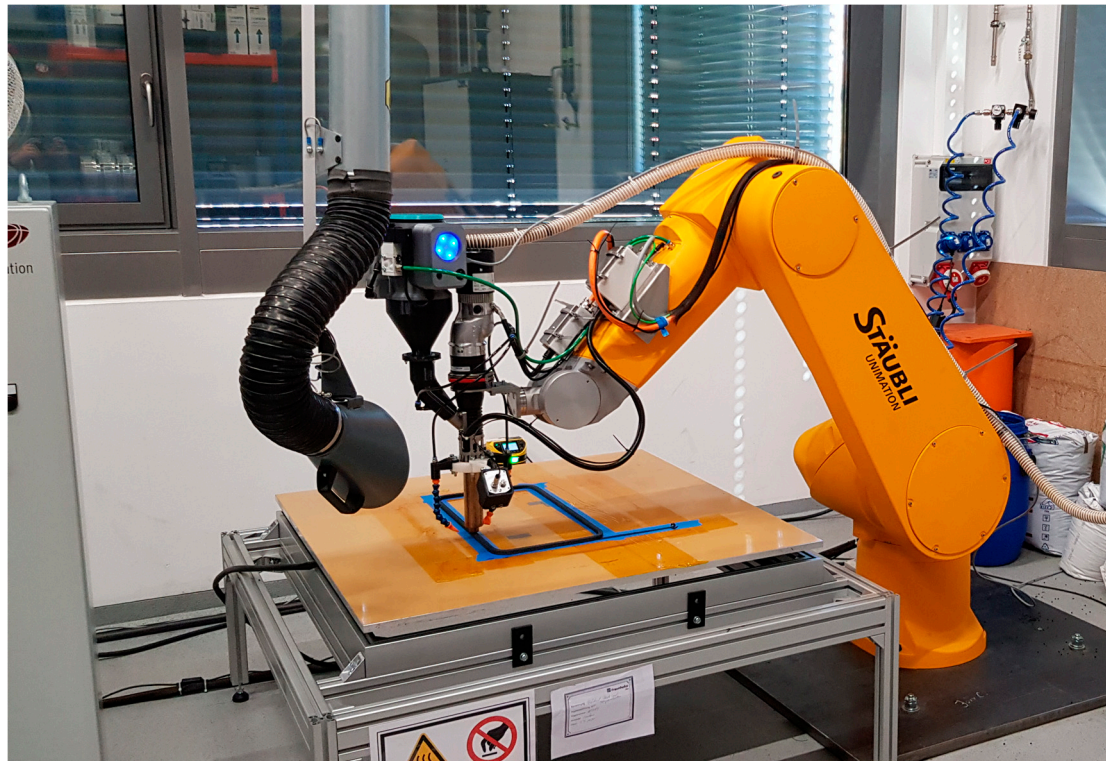
Figure 1. Fused granular fabrication unit used to produce fiber-reinforced polyamide test structures.
