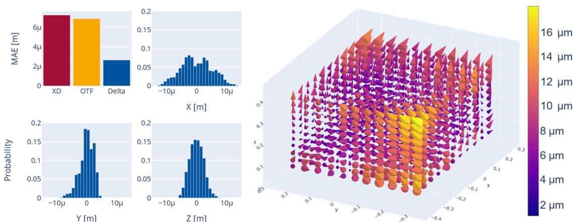
**Figure 9.** (Top left): Mean absolute error on a regular grid calculated using error table data from XD Laser, OTF calibration with a RBM, and the MAE of the delta between both. Please note the magnitude of errors. (Left): Histograms showing relative probability for volumetric error deviations in X/Y/Z on a grid between XD Laser measurement and OTF calibration. (Right): Difference visualized as cone plot on the regular grid (grid axis unit: [m]).
