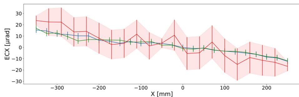
**Figure 8.** ECX error. Blue/green are forward/backward values for API XD Laser measurements with respective error bars computed from values over five measurement runs. Red is OTF laser tracker measurements with respective computed uncertainty area.
