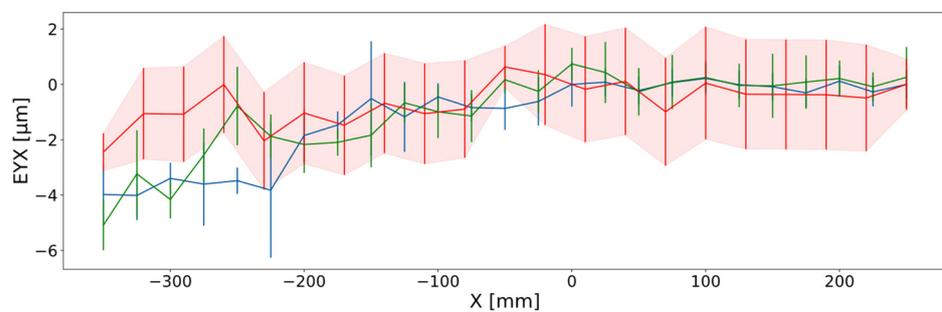
**Figure 7.** EYX error. Blue/green are forward/backward values for API XD Laser measurements with respective error bars computed from values over five measurement runs. Red is OTF laser tracker measurements with respective computed uncertainty area.
