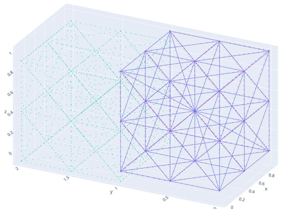
**Figure 1.** Simulated exemplary OTF calibration path (blue, continuous) and simulated laser tracker measurements points (green). Note the shift and rotation (by 90°) between both shapes demonstrating the different coordinate systems of laser tracker and machine. Red points show simulated measurement points after rough alignment.
