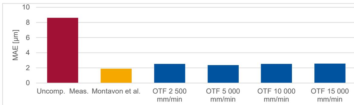
**Figure 5.** Volumetric error prediction comparison with different methods on a random set of points. Uncomp. Meas. shows the mean absolute error (MAE) vector length over all reference points. Montavon et al. [14] shows the mean absolute error between the measured points and their prediction using standstill calibration method. The OTF bars show MAE for OTF calibration with different velocities.
