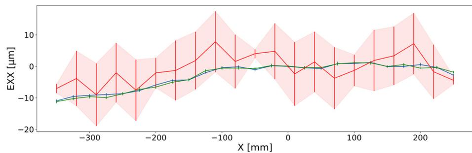
**Figure 6.** EXX error as an exemplary positioning error. Blue/green are forward/backward values for API XD Laser measurements with respective error bars computed from values over five measurement runs. Red is OTF laser tracker measurements with respective computed uncertainty area.
