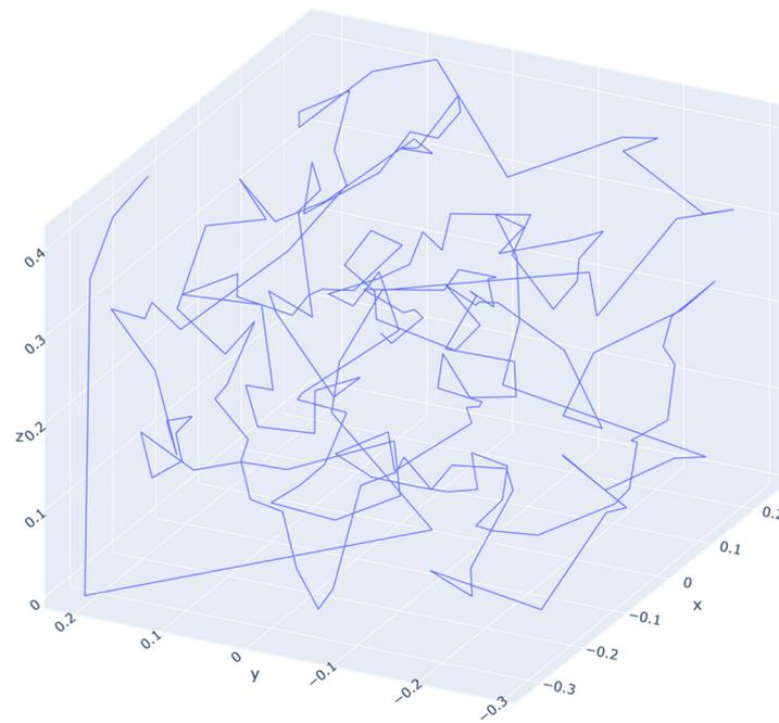
**Figure 2.** Reference trajectory to compare standstill laser tracker calibration with OTF calibration on (grid axis unit: [m]).
