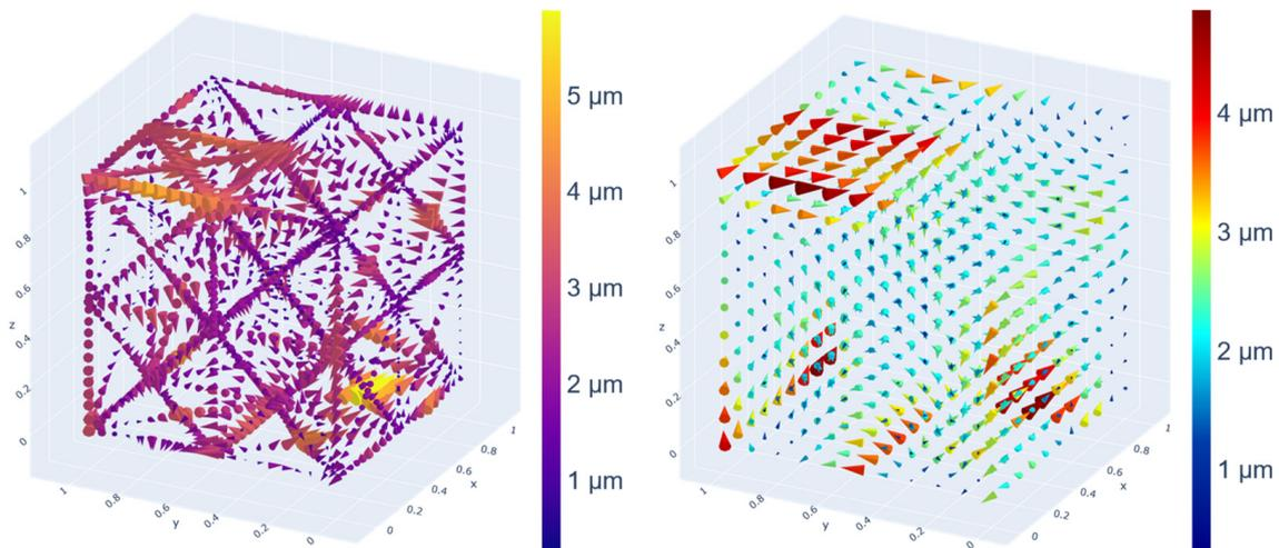
**Figure 4.** (Left side) shows simulated residual deviations on path, right shows residual volumetric errors on a regular grid (grid axis unit: [m]). Larger deviations seem to occur in areas of ambiguity: residuals generally larger in path direction can be seen on the (left side).
