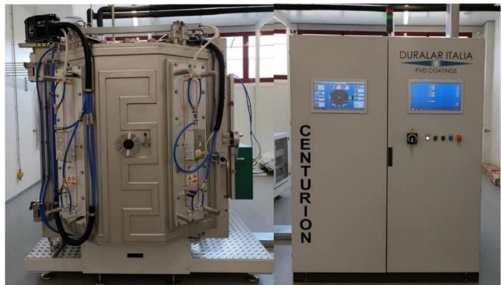
**Figure 5.** Photograph of Duralar Centurion system employed for PE-CVD deposition.
