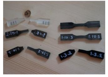
Figure 10. Dog-bone tensile specimens before and after tensile test.
