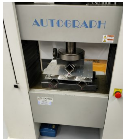
Figure 11. Three-point bending test to examine mechanical properties of assembled truss core panel.
