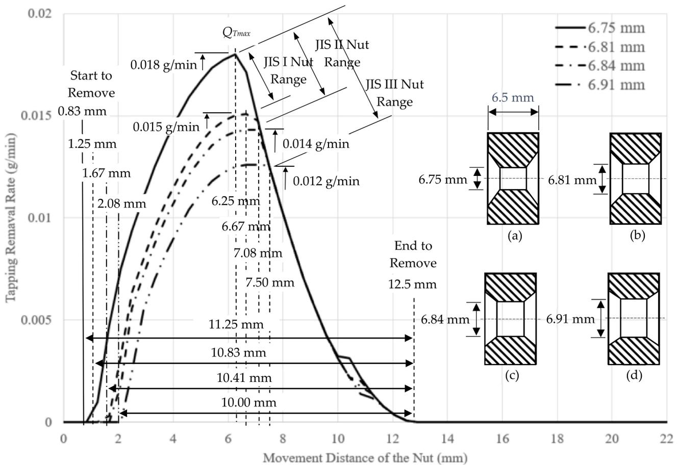
**Figure 6.** The tapping removal amount in different hole size: (a) 6.75 mm; (b) 6.81 mm; (c) 6.84 mm; (d) 6.91 mm.
