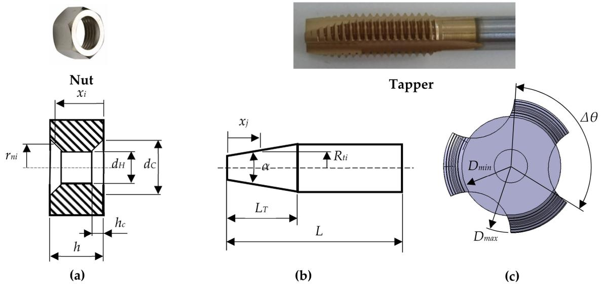
Figure 3. Parameters: (a) nut; (b) side view of tapper; (c) front view of tapper.
