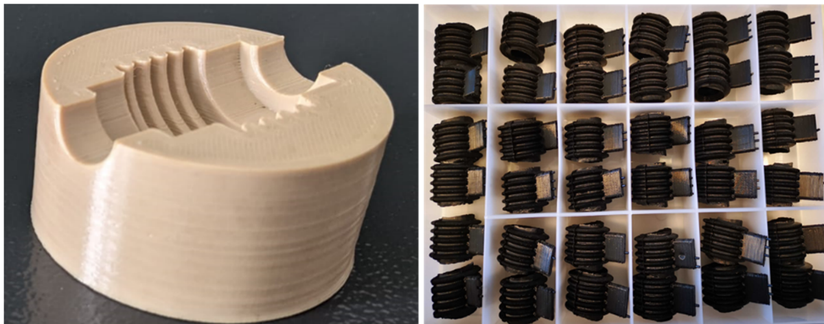
Figure 1. PEEK Mold Half (left); Injection-molded rubber parts (right).
