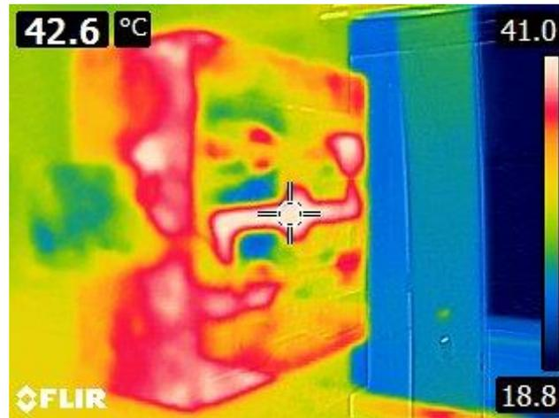
**Figure 2.** Temperature profile of the steel mould after 23 shots.
