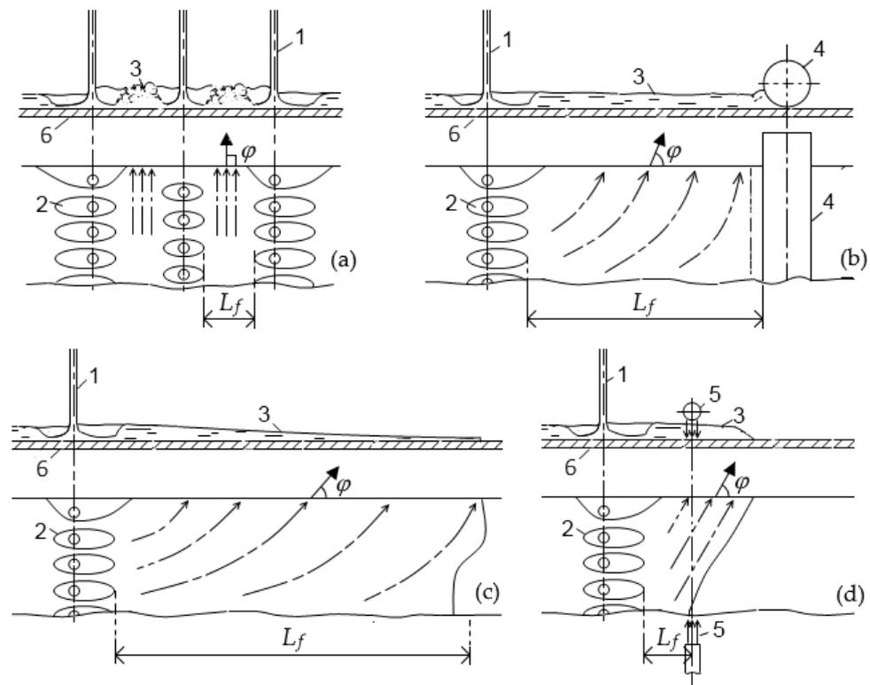
**Figure 6.** Different types of subcritical flow zone (“water layer”): (a) clamped, (b) bounded, (c) open and (d) shifted. Designations: 1—jet, 2—supercritical flow area, 3—water layer, 4—roll, 5—separator.  $L_f$  is the length of the water layer;  $\varphi$  is the runoff angle.
