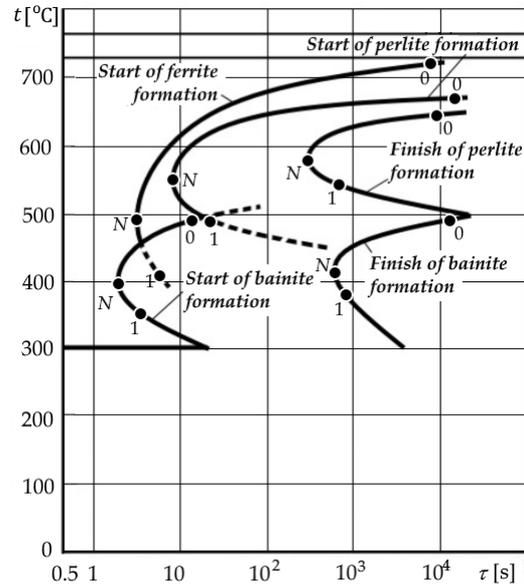
**Figure 9.** Example of a TTT-diagram showing a 3-point approximation scheme. Diagram shows the reference points taken in the approximation for each C-curve: 0—upper, N—“nose”, 1—lower.
