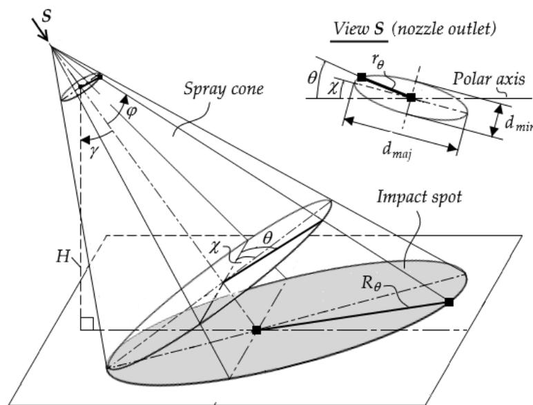
Figure 3. Schematic explaining the designations used in calculating the dimensions of the impact spot of the spray jet.
