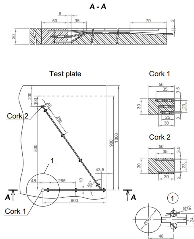
Figure 12. Thermocouple embedding scheme (dimensions are in mm). Of the five channels prepared, four were used in each test plate (details in the text).
