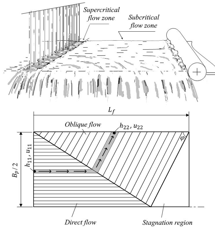
**Figure 7.** Schematic explaining the basic idea of calculating the parameters of the subcritical water flow zone by conventionally dividing this zone into three regions: direct flow, oblique flow and stagnation region. The arrows show the direction of water flow in the median streamline. The designations are in the text.
