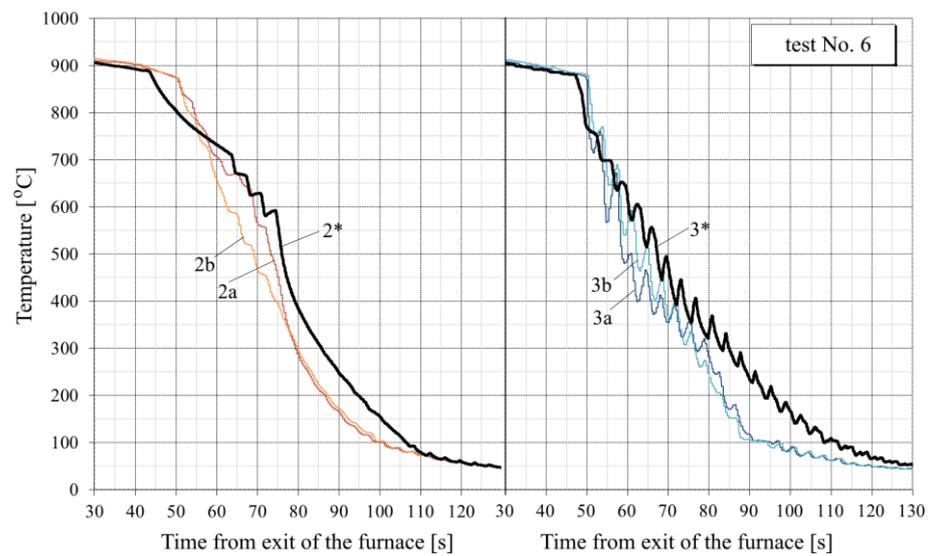
Figure A4. Graphs of cooling in test No. 6. Numbers without an asterisk denote experimental curves according to the thermocouple data: 2a—at the top in the middle of the width; 2b—at the top at the edge, 3a—at the bottom in the middle of the width; 3b—at the bottom at the edge. Numbers with one asterisk indicate calculated curves for the corresponding control points across the thickness of the plate: 2\*—at a depth of 3 mm from the top surface; 3\*—at a depth of 2.5 mm from the bottom surface.
