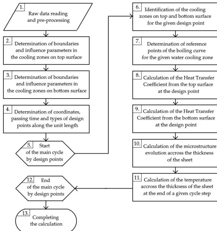
**Figure 2.** Block diagram of the cooling model.
