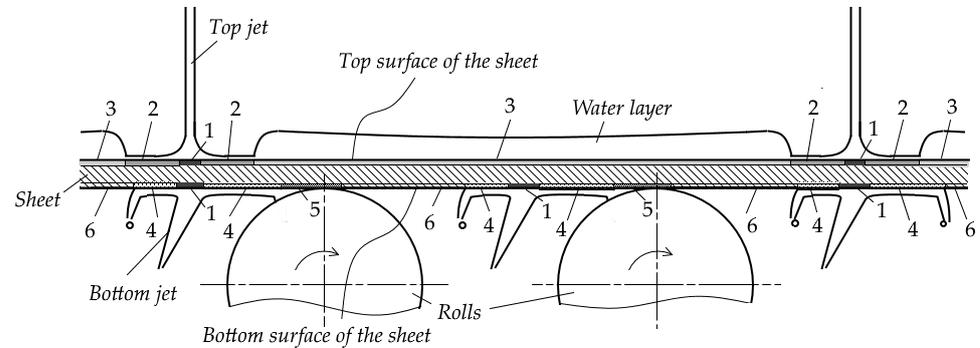
**Figure 1.** Schematic explaining the types of cooling zones considered in the model (indicated by numbers): 1—jet impingement; 2—supercritical flow on the top surface; 3—subcritical flow on the top surface; 4—parallel flow on the bottom surface; 5—contact with a roll; 6—air cooling.
