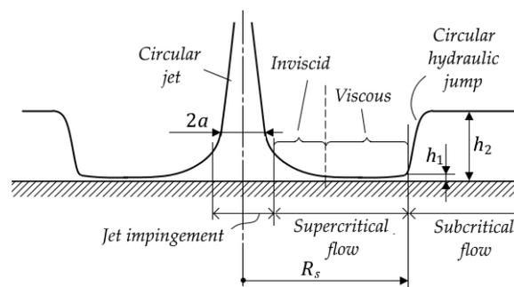
**Figure 4.** Schematic of the flow of a circular liquid jet on a horizontal plate with the formation of a circular hydraulic jump. The zones of jet impingement, and supercritical and subcritical flow are shown. Supercritical flow zone is conventionally divided into two regions: inviscid and viscous.
