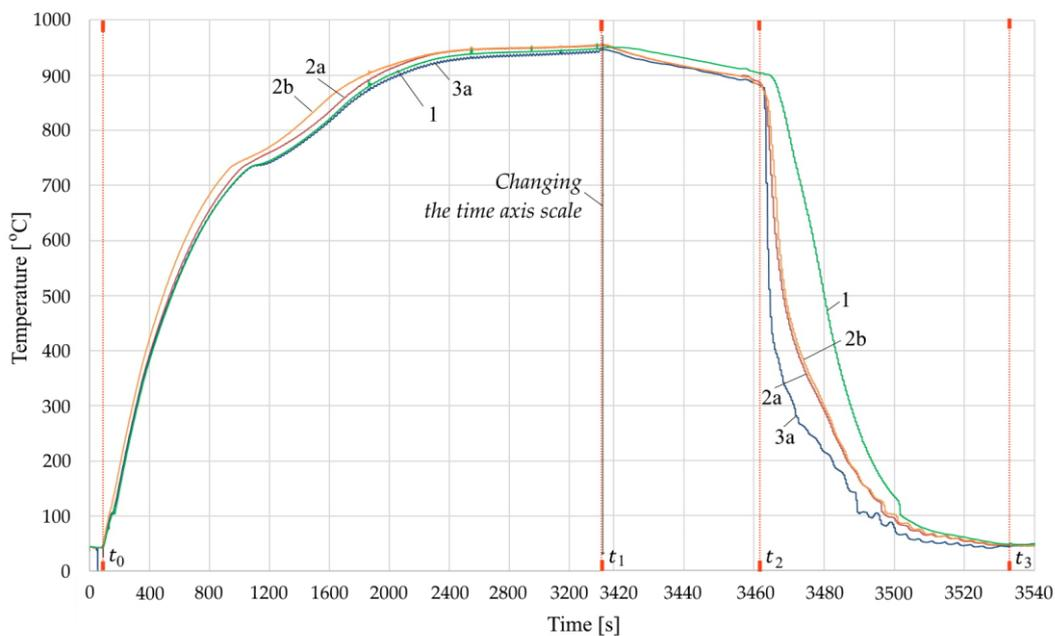
Figure 13. Plots of temperature changes, measured using thermocouples in test No. 2 during heating and cooling. Designations of the curves: 1—at the center of the thickness in the middle of the plate width; 2a—at the top in the middle of the width; 2b—at the top at the edge; and 3a—at the bottom in the middle of the width. Designations of the key moments of time:  $t_0$ —entry into the furnace;  $t_1$ —exit from the furnace;  $t_2$ —entry into the first zone of RQM;  $t_3$ —exit from RQM.
