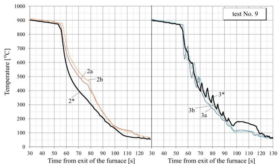
Figure A7. Graphs of cooling in test No. 9. The notations are the same as in Figure A4.
