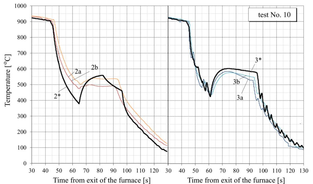
Figure 16. Graphs of cooling in test No. 10. Numbers without an asterisk denote experimental curves according to the thermocouple data: 2a—at the top in the middle of the width; 2b—at the top at the edge; 3a—at the bottom in the middle of the width; 3b—at the bottom at the edge. Numbers with one asterisk indicate calculated curves for the corresponding control points across the thickness of the plate: 2\*—at a depth of 3 mm from the top surface; 3\*—at a depth of 2.5 mm from the bottom surface.
