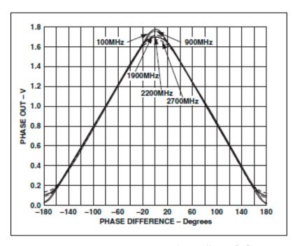
Figure 7. Phase Output vs. Input Phase Difference [23].
