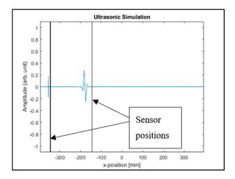
**Figure 1.** A-scan image of simulation.
