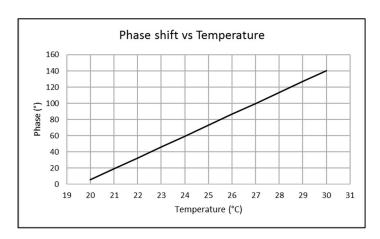
Figure 5. Phase-shift vs. temperature for 15mm steel.
