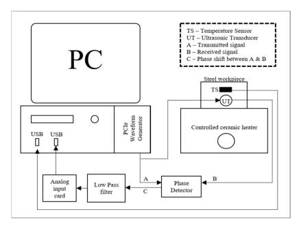
Figure 6. Ultrasonic phase-shift experimental setup.
