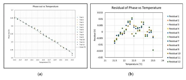
Figure 10. Results of 21.5 to 23.5 °C range in 0.1 °C steps (a) Phase output vs. temp; (b) Residual plot.
