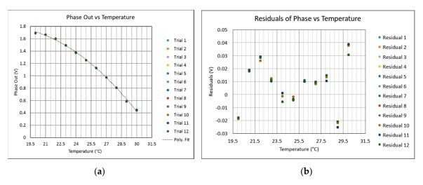
**Figure 9.** Results of 20 to 30 °C range in 1 °C steps (a) Phase output vs. temperature; (b) Residual plot.
