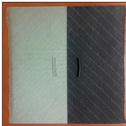
**Figure 2.** Plaques with net epoxy (**left**) and 1 wt% graphene addition to epoxy (**right**) and their respective epoxy.
