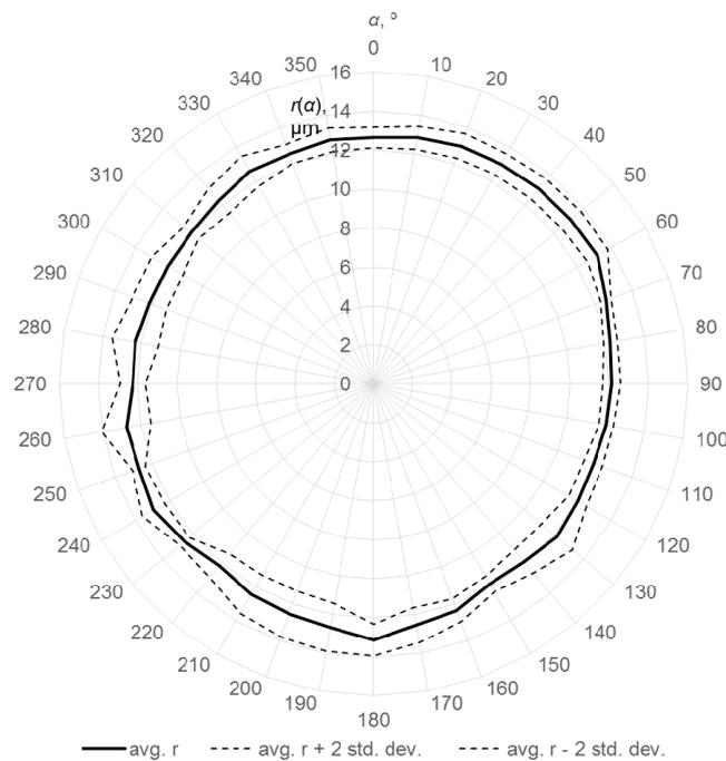
**Figure 4.** Results obtained in the laboratory for strain gauge probe with a 100 mm stylus.
