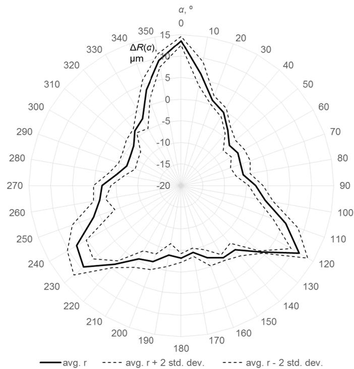
**Figure 6.** Results obtained on the machine tool for ultra-compact touch-trigger probe with 100 mm stylus, for measurement speed equal to 150 mm/min.
