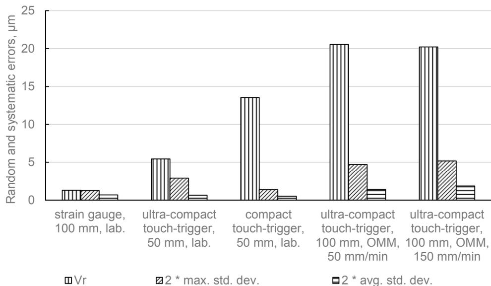
Figure 7. Random and systematic errors share vs. probe type and stylus length.
