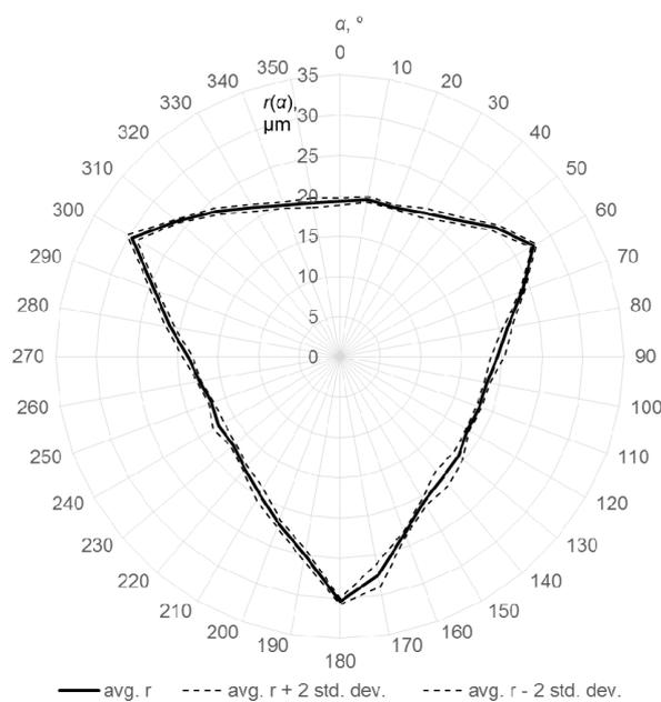
Figure 3. Results obtained in the laboratory for compact touch-trigger probe with a 50 mm stylus.
