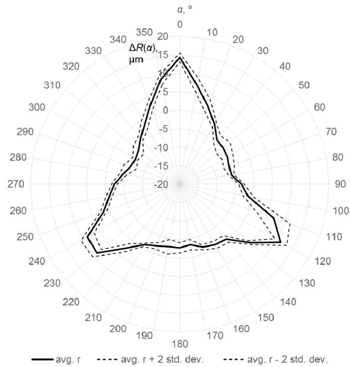
**Figure 5.** Results obtained on the machine tool for ultra-compact touch-trigger probe with 100 mm stylus, for measurement speed equal to 50 mm/min.
