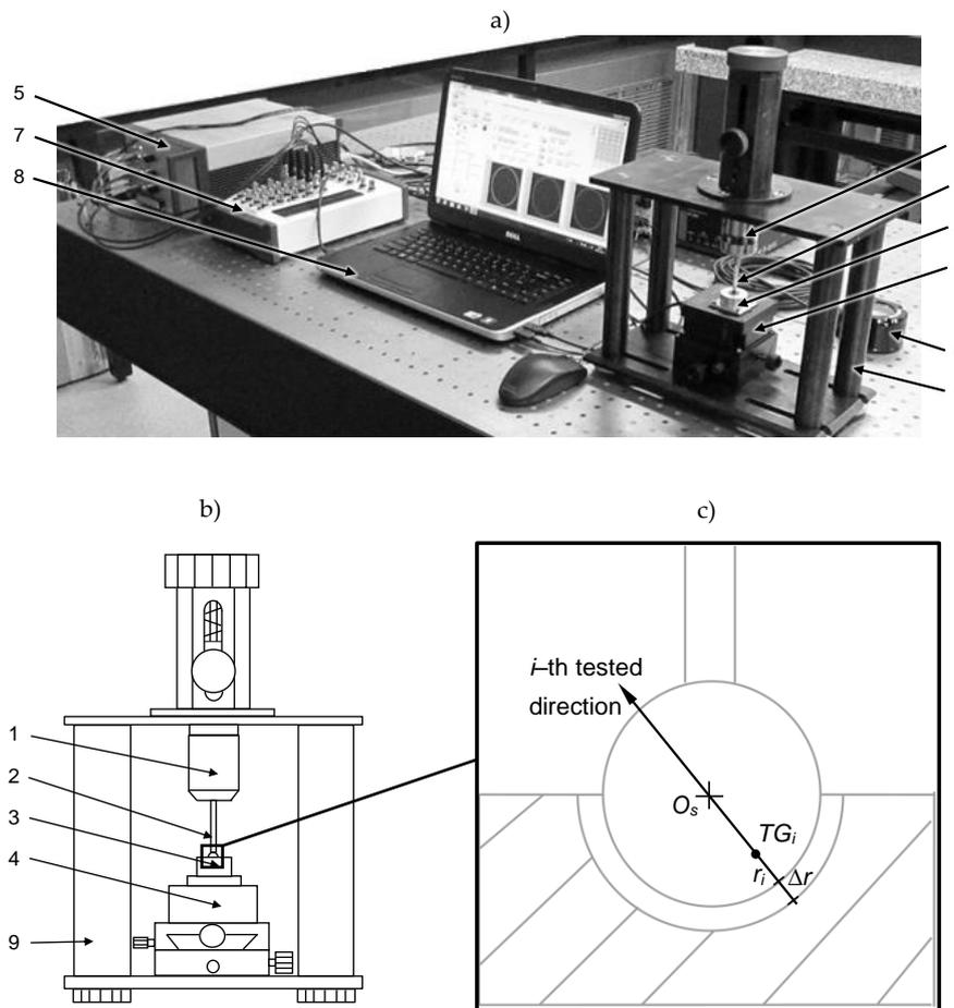
**Figure 1.** Setup for probe testing: (a) view, (b) scheme of the mechanical unit of the setup, and (c) detail—stylus tip placed inside of the inner hemisphere master artefact: 1—tested probe, 2—stylus tip, 3—master artefact, 4—3-axial piezostage, 5—piezostage controller, 6—probe's interface receiver, 7—DAQ card, 8—PC, 9—frame.
