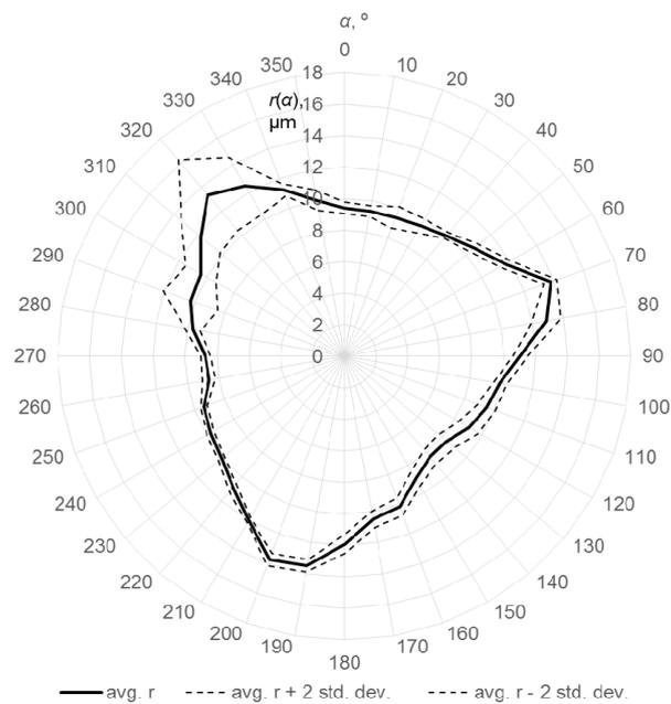
Figure 2. Results obtained in the laboratory for ultra-compact touch-trigger probe with a 50 mm stylus.
