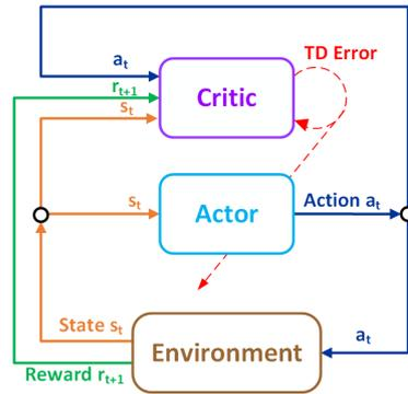
**Figure 4.** Actor–critic architecture showing that the actor receives the state and produces the actions. The critic network receives the state and the actions produced by the actor and produces a state value to criticize the action made by the actor.
