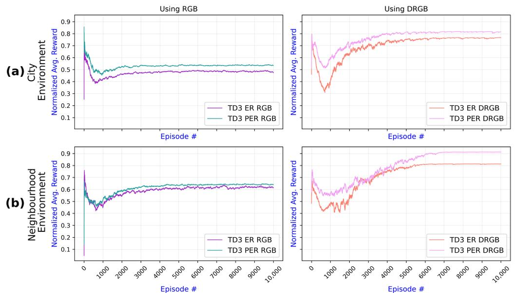
**Figure 12.** Comparison of TD3 algorithm results showing the impact of PER over ER in two navigation environments: (a) In the city environment, incorporating PER enhances performance with both RGB and DRGB image inputs. (b) Results for the neighborhood environment have a similar pattern but slightly later stabilization.
