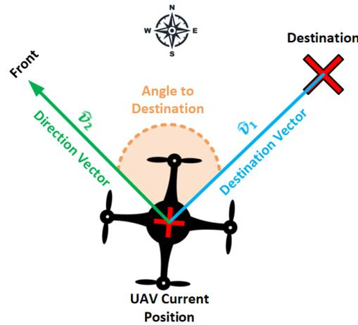
**Figure 2.** UAV orientation angle with respect to the destination point. The angle is measured using two vectors: the destination vector  $\hat{v}_1$ , which points from the UAV's current location to the destination point, and the direction vector  $\hat{v}_2$ , which points in the forward direction of the UAV.
