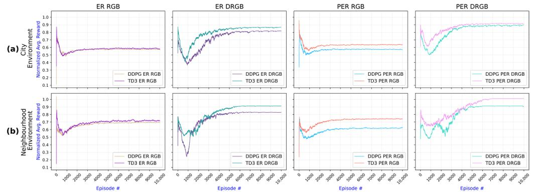
**Figure 8.** Comparative analysis of DDPG and TD3 algorithms across the four experiments: ER with RGB, ER with DRGB (depth images), PER with RGB, and PER with DRGB. Each row presents the results for one environment: (a) Results for the city environment show that TD3 with PER and DRGB achieves higher average reward than the other approaches. (b) Results for the neighborhood environment confirm that TD3 using PER combined with DRGB yields better results.
