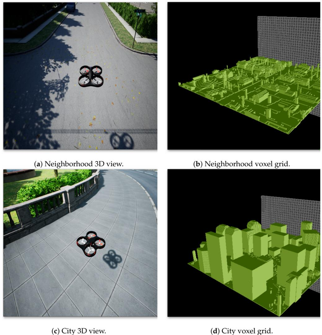
**Figure 6.** An overview of the two simulation environments used for the UAV navigation experiments summarizing spatial layout and obstacle distribution for illustrative purposes. Panels (a,b) show the neighborhood’s 3D view and voxel grid, respectively. Panels (c,d) show the city block’s 3D view and voxel grid, respectively.
