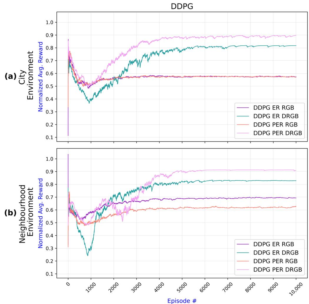
**Figure 10.** Comparison of DDPG algorithm results across two environments with different setups—ER with RGB, ER with DRGB, PER with RGB, and PER with DRGB: (a) Results for the city environment show that inclusion of DRGB has a higher impact than replacing ER with PER. (b) Results for the neighborhood environment confirm that PER and depth images (DRGB) improve navigation.
