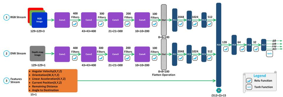
**Figure 5.** DRL neural network architecture showing three streams for processing state information: (1) RGB stream, (2) DMI stream, and (3) features stream. The concatenation layer FC4 fuses the data received from the three streams.
