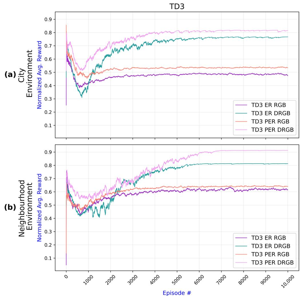
**Figure 9.** Comparison of TD3 algorithm results across two environments with different setups—ER with RGB, ER with DRGB, PER with RGB, and PER with DRGB: (a) Results for the city environment show that inclusion of DRGB has a higher impact than replacing ER with PER. (b) Results for the neighborhood environment confirm that PER and depth images (DRGB) improve navigation.
