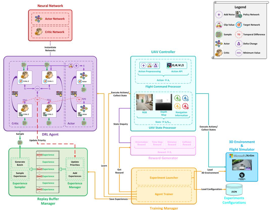
**Figure 3.** VizNav framework showing interactions between various modules using the TD3 algorithm with PER. Loading the configurations and 3D environment helps to execute various experiments depending on the needs.
