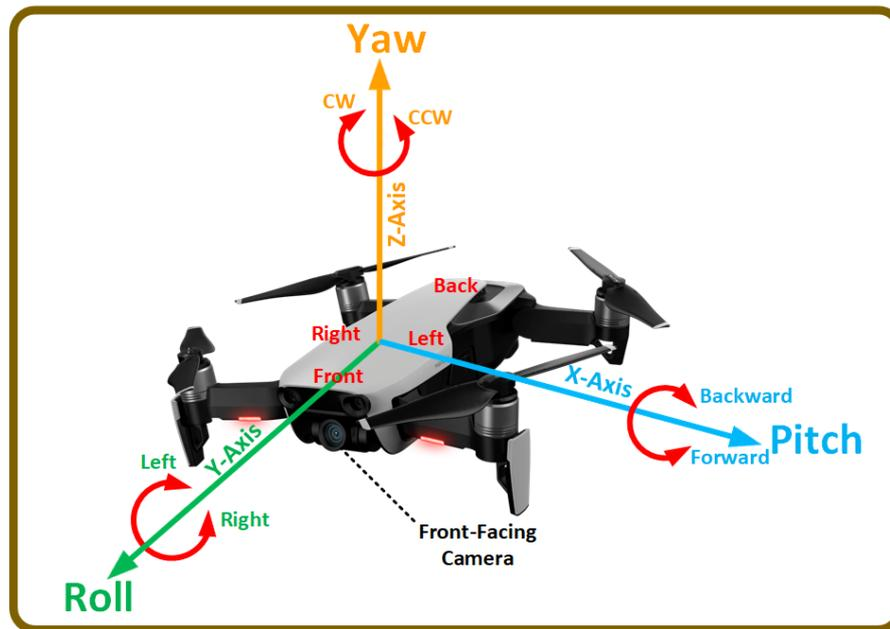
**Figure 1.** The UAV control mechanism demonstrates regulating the UAV's movement through the rotation angle around three axes—pitch, roll, and yaw—while the throttle adjusts the engines' thrust. Rotation around the roll axis, highlighted in green, directs the UAV left or right. Rotation around the pitch axis, shown in blue, moves the UAV forward or backward. Rotation around the yaw axis, depicted in orange, enables clockwise (CW) or counterclockwise (CCW) rotation.
