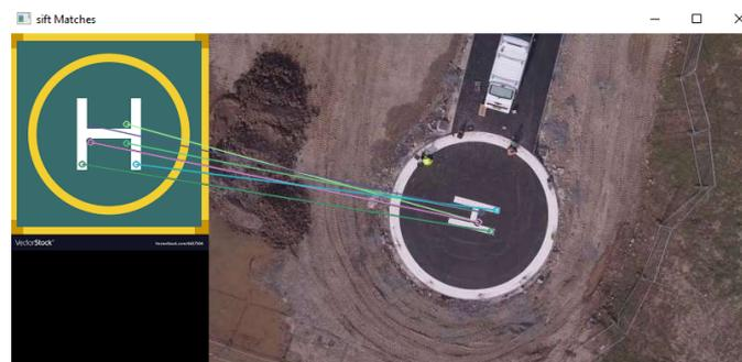
**Figure 12.** Matching of Reference and Target image using SIFT.
