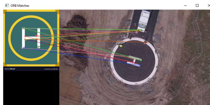
**Figure 13.** Matching of Reference and Target image using ORB.
