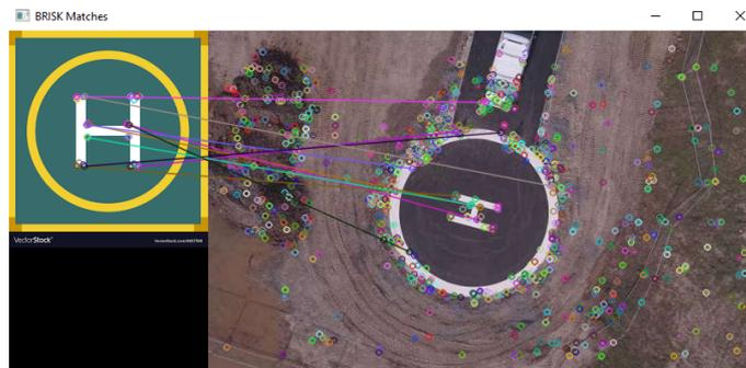
**Figure 15.** Matching of Reference and Target image using BRISK.
