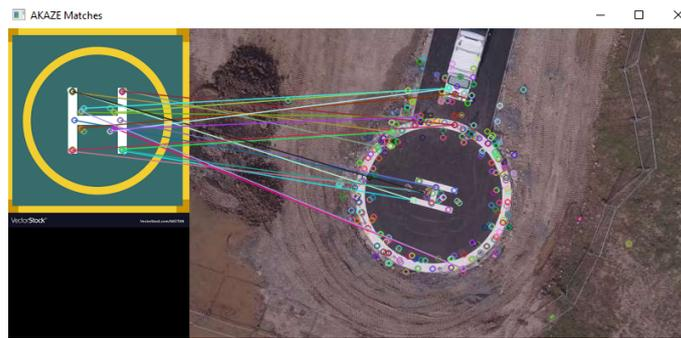
**Figure 14.** Matching of Reference and Target image using AKAZE.
