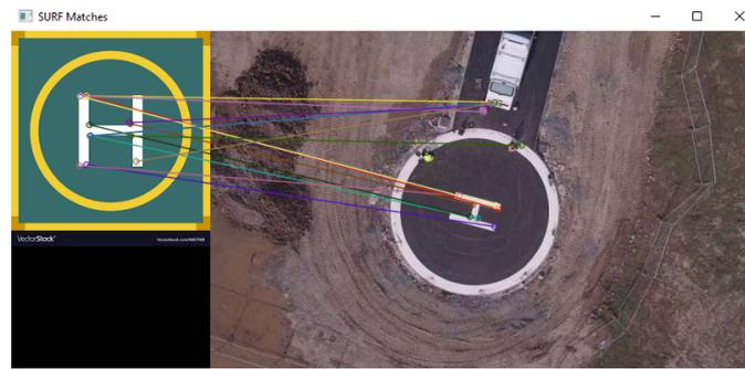
**Figure 11.** Matching of Reference and Target image using SURF.
