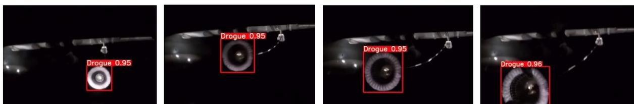
Figure 13. Drogue detection results under low-light conditions.
