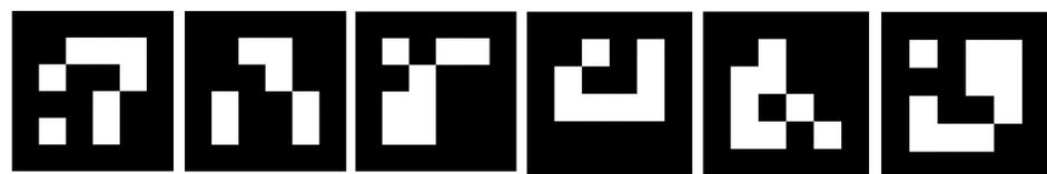
**Figure 2.** The patterns of Augmented Reality University of Cordoba (ArUco) marker. The sequence of marker patterns’ ID from left to right is 0~5.
