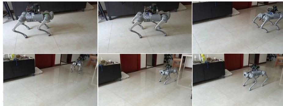
**Figure 3.** Mapping process of the quadruped robot with LiDAR.
