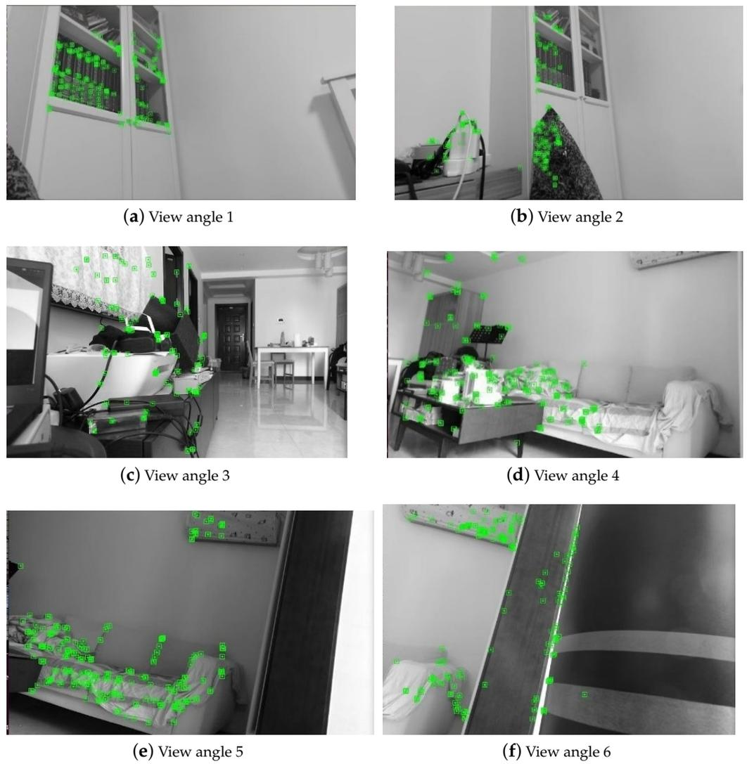
**Figure 5.** The successful tracking outcome achieved with ORB-SLAM2: feature points are labeled and a point cloud map can be generated.
