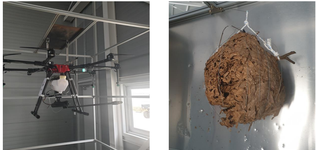
Figure 6. Performance test of the spraying and perforation devices: (left) UAV exterminator fixed to aluminum profile holder and (right) nest condition after experiment.
