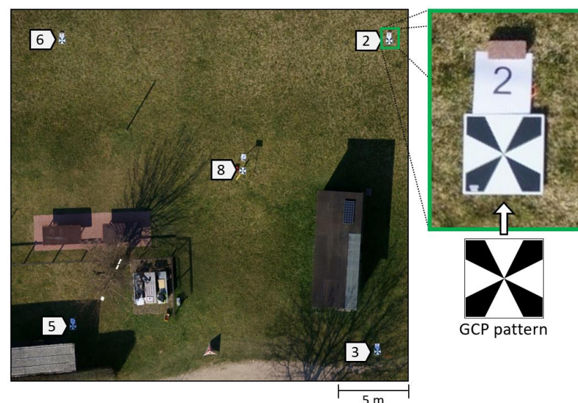
Figure 1. (Left) Study area with five placed GCP numbered 2, 3, 5, 6, and 8. (Top right) Image section of GCP from nadir flight 30 m above the ground with 4.2 mm GSD. (Bottom right) Eight-fold GCP design pattern.
