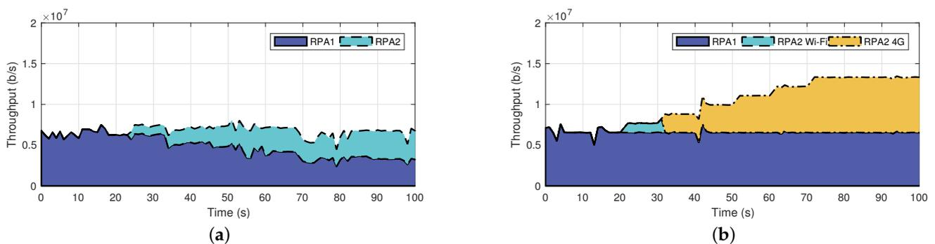
**Figure 6.** Load balancing experiment. (a) No load balancing (traffic received at the RPS); (b) load balancing (traffic received at the RPS).
