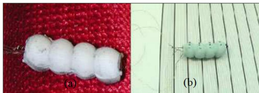
**Figure 17.** View of robotic earthworm design using shape memory alloy locomotion technology (a) with and (b) without micro-legs [29].
