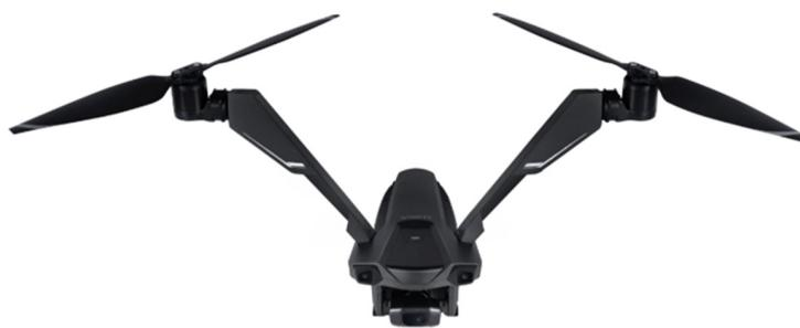
**Figure 29.** V-Copter Falcon by Zero Zero Robotics with two tilting rotors [42].
