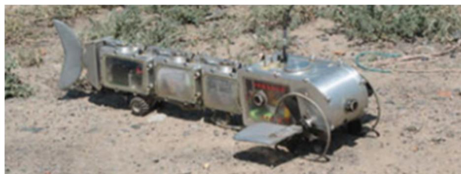
**Figure 23.** Mechanism design of AmphiRobot-II; prototype of the amphibious robot in the field test [36].
