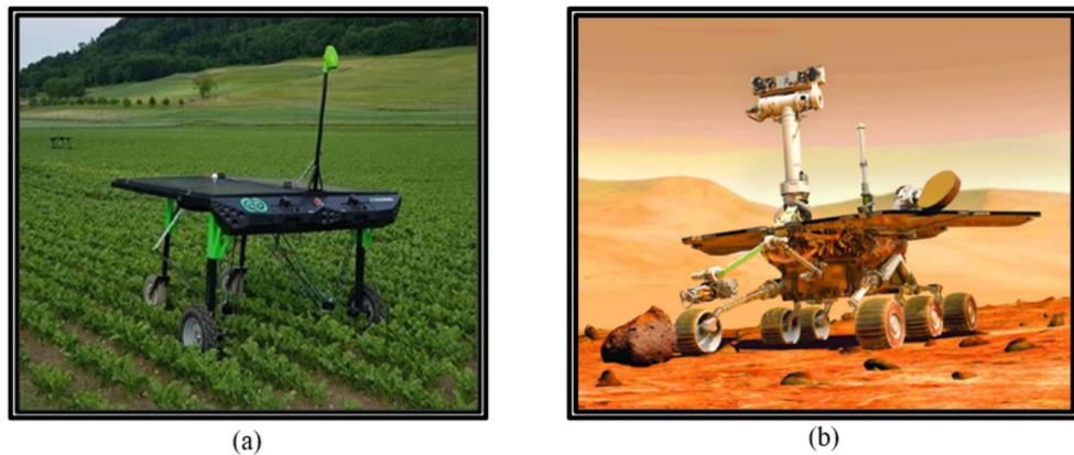
**Figure 2.** Examples of wheeled UGVs with specialized functionalities: (a) four-wheeled UGV drives through seedlings, picking weeds between rows [13]; (b) six-wheeled UCV traverses Mars' surface.
