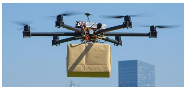
**Figure 33.** Hexacopter drone used for package delivery [46].
