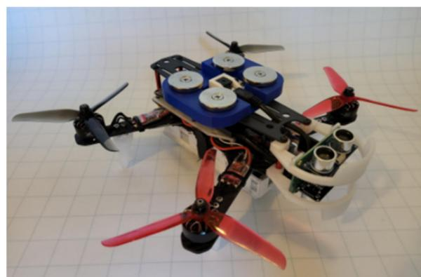
**Figure 32.** Semi-autonomous precision-docking quadcopter constructed from a racing drone frame with custom sensors and flight controllers [45].
