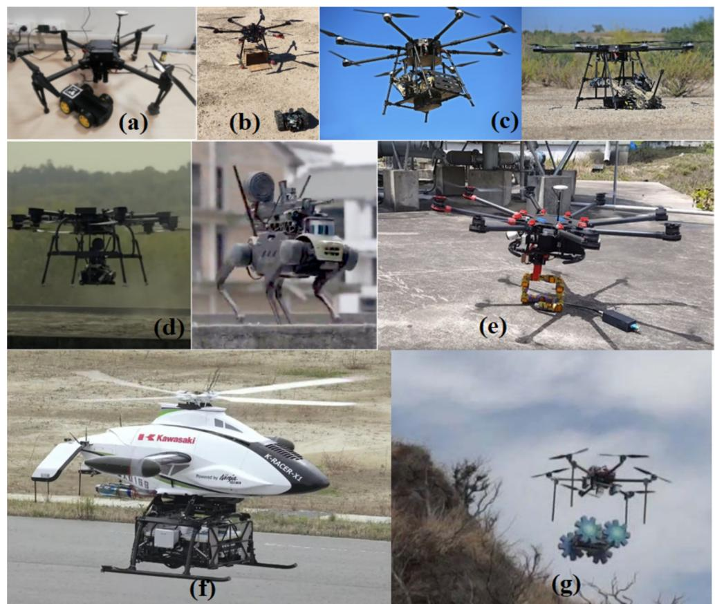
**Figure 53.** View of (a) drone transporting a ground robot [142], (b) team of autonomous drones and UGVs for civil infrastructure inspection [143], (c) a drone that can carry a Micro Tactical Ground Robot (MTGR) [144], (d) drone deploying a quadrupedal unmanned ground vehicle [145], (e) a drone that can carry a snake robot for accident monitoring [146], (f) autonomous helicopter which transport a cargo robot [147], and (g) a robotic systems for volcano exploration [148].
