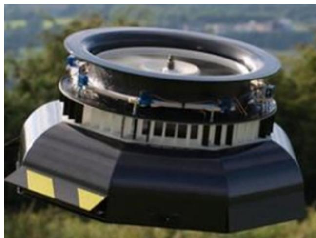
**Figure 28.** Aesir drone utilizing a single rotor and the Coandă effect for flight [41].
