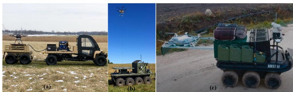
**Figure 46.** Views of tethered drones deployed by military UGVs [92].
