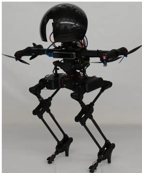
**Figure 40.** LEONARDO, the walking, hopping, flying drone, is modeled after birds that can both fly and hop in order to navigate telephone lines [71].
