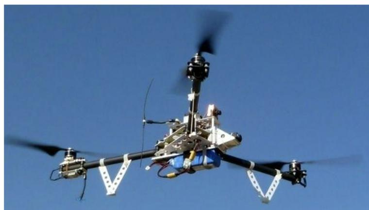
**Figure 30.** Tri-rotor drone in flight [43].
