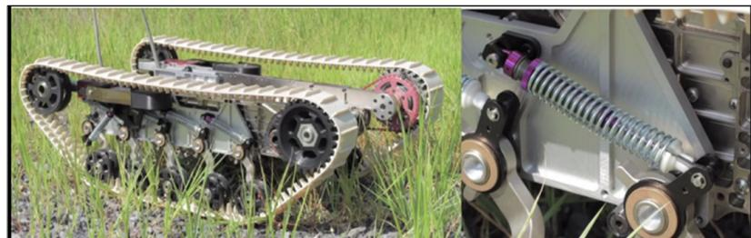
**Figure 7.** The spring-loaded suspension between tank track drives and supports [19].
