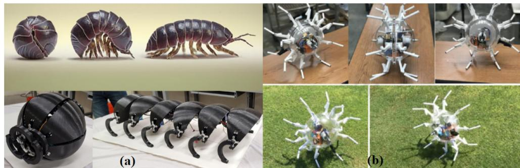
**Figure 21.** View of (a) rolling isopod-based robot demonstrating the conglobulation process [34] and (b) golden-wheel-inspired rolling robot [24].
