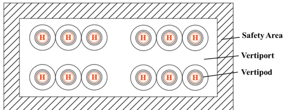
Figure 15. Vertipod layout on building roof.
