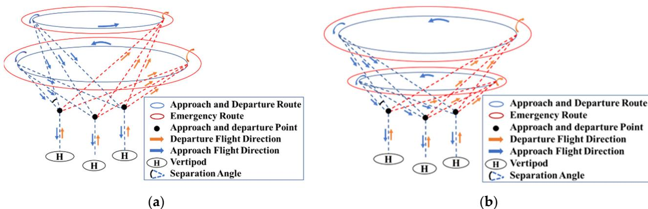
Figure 17. Terminal area approach and departure layout. (a) Layout one, (b) Layout two.
