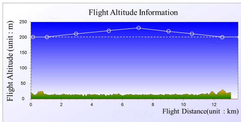
**Figure 24.** Altitude profiles of collision avoidance rule simulation.
