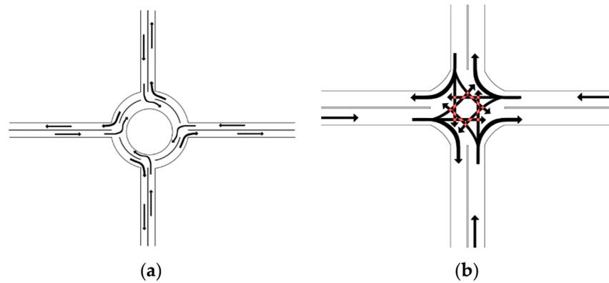
Figure 7. Turning diagram. (a) Circular intersection, (b) cross intersection.
