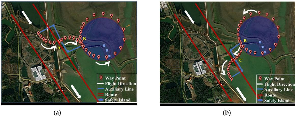
**Figure 22.** Simulation trajectory diagram of eVTOL aircraft leaving or entering route. (a) Leaving route, (b) entering route.
