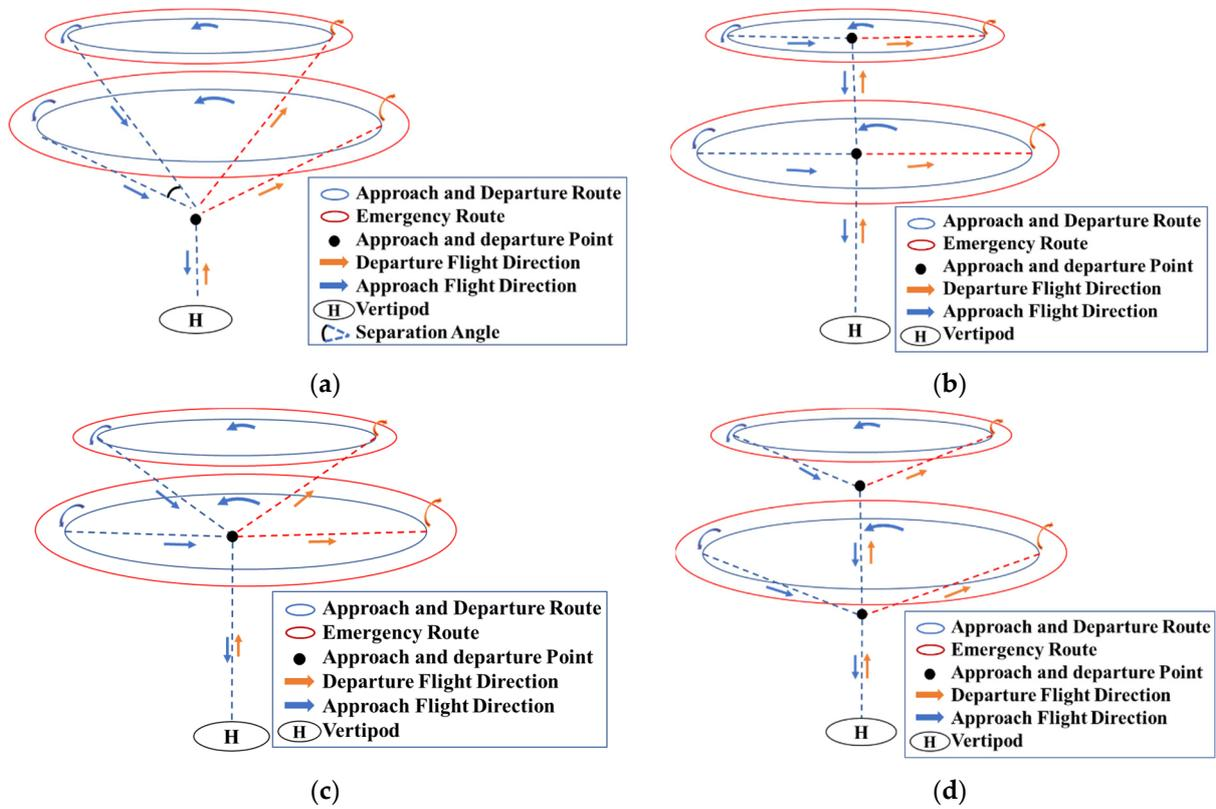
Figure 18. Number and location of approach and departure positioning points. (a) Layout one, (b) Layout two, (c) Layout three, (d) Layout four.
