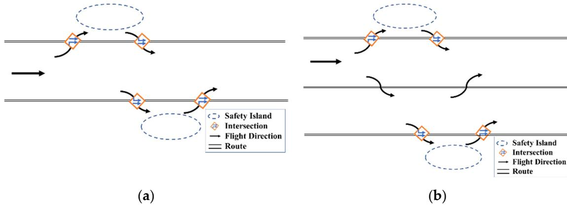
Figure 5. eVTOL aircraft entering or leaving routes at different stages. (a) Early stage, (b) middle stage.
