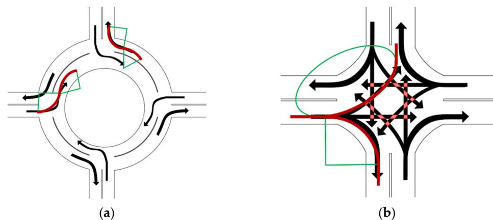
Figure 8. Turning diagram. (a) Circular intersection, (b) cross intersection.
