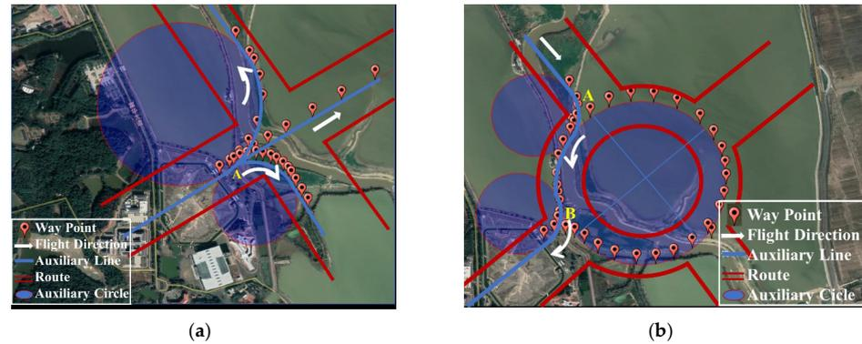
Figure 25. Turning rule simulation. (a) Cross intersection, (b) roundabout intersection.
