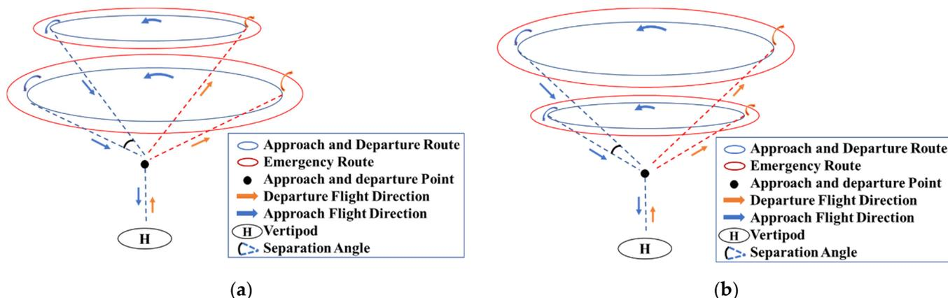
Figure 16. Terminal area approach and departure layout. (a) Layout one, (b) Layout two.
