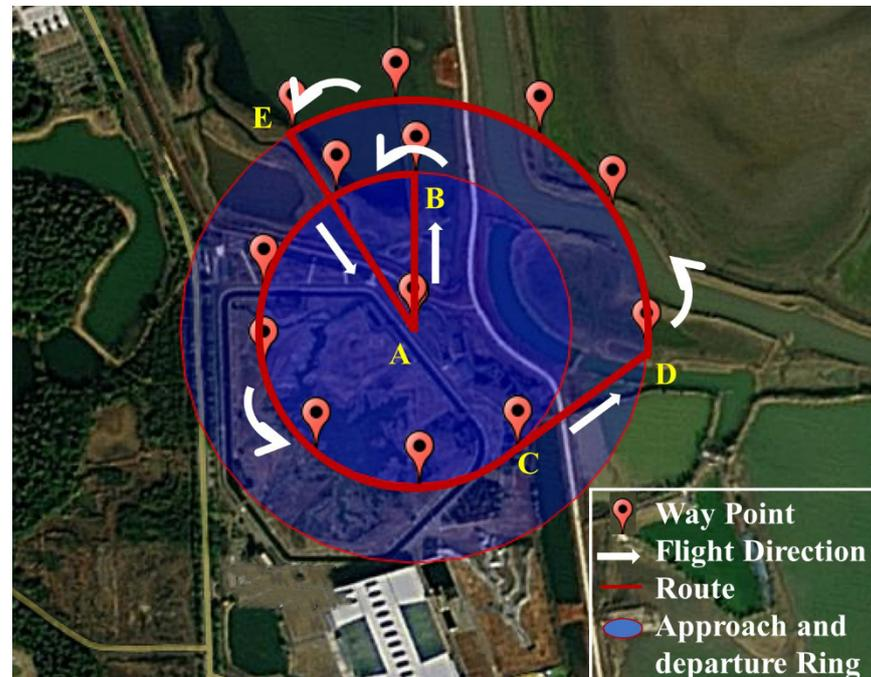
Figure 27. Terminal area approach and departure simulation.
