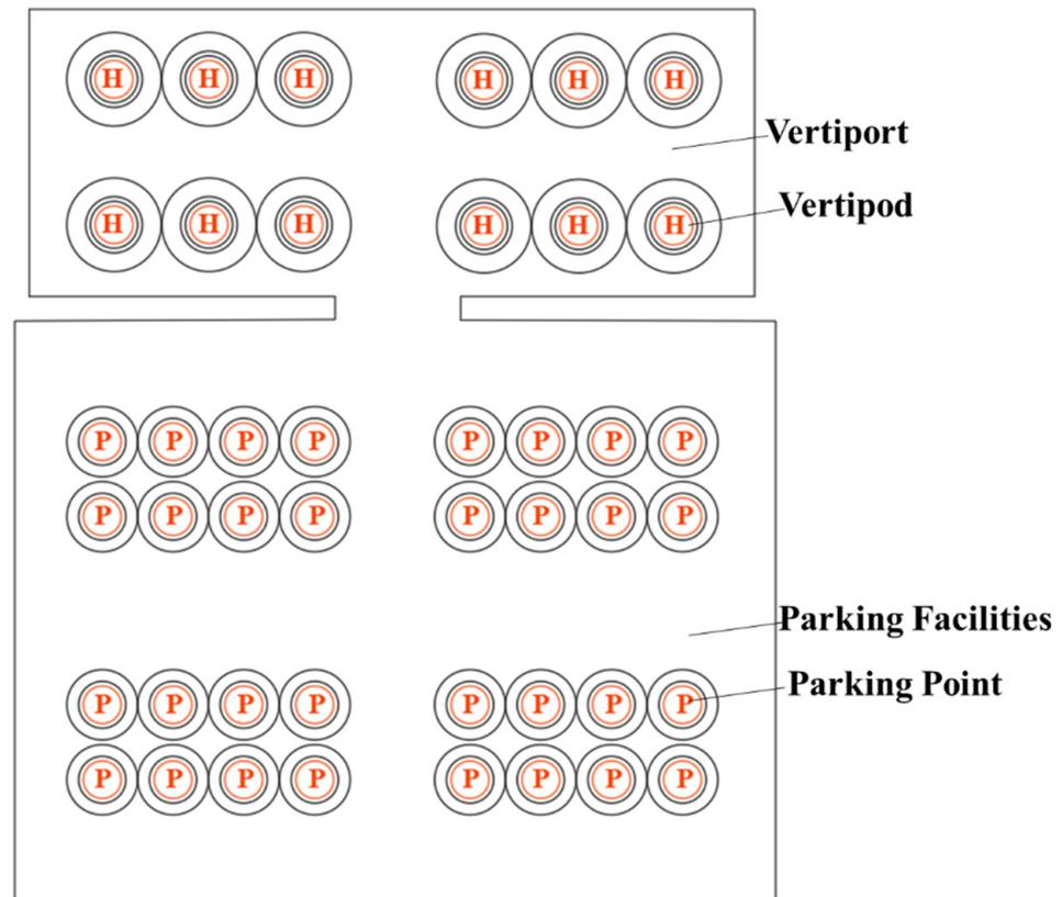
Figure 14. Vertipod layout on open ground or transportation hub.
