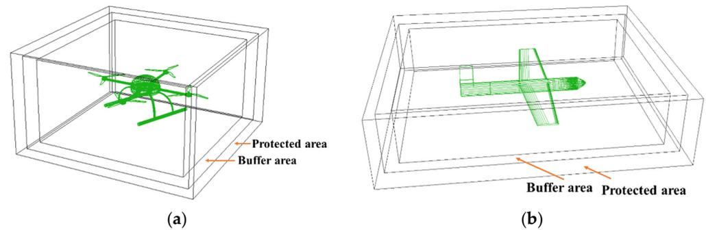
**Figure 4.** Space-time capsule. (a) Multi-rotor eVTOL aircraft, (b) fixed-wing eVTOL aircraft.
