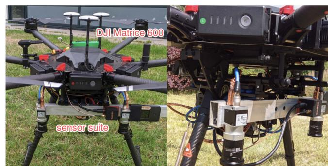
**Figure 3.** Sensor suite and the mini computer mounted on the drone.
