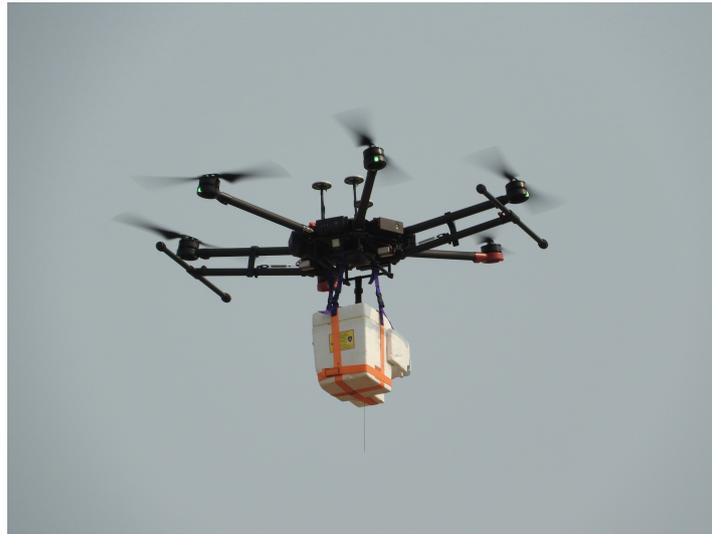
**Figure 1.** DJI M600 in flight with an ozonesonde and radiosonde attached below.
