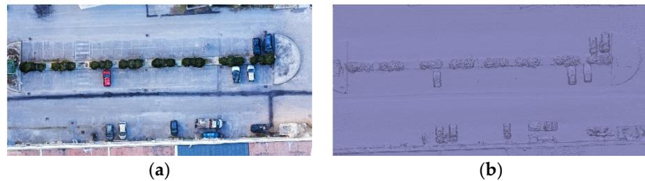
**Figure 7.** SfM reconstruction using super-resolution image dataset: (a) Model shaded view; (b) solid mesh view.
