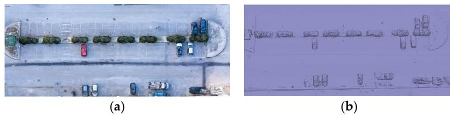
**Figure 6.** SfM reconstruction using low-resolution image dataset: (a) model shaded view; (b) solid mesh view.
