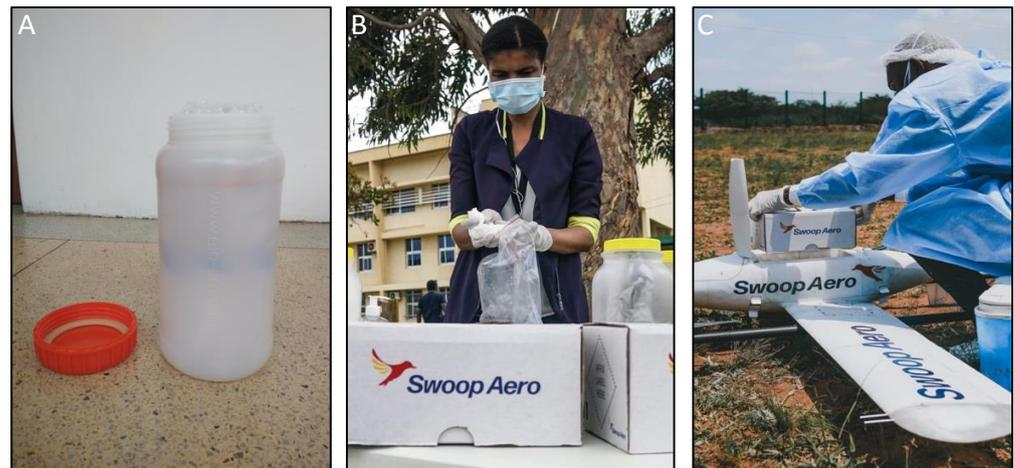
**Figure 1.** Schematic of sample packaging. (A) Ridged waterproof container; (B) Swoop Aero cargo box; (C) Placement of cargo box in aircraft.
