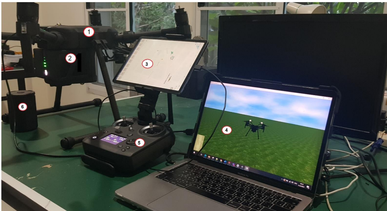
Figure 3. Drone ground station consisting of (1) drone, (2) rechargeable battery, (3) tablet to program the drone, (4) drone server, (5) the remote control of the drone, and (6) battery charger.
