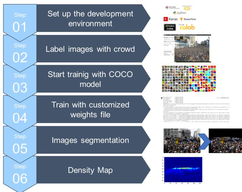
**Figure 7.** Steps of the development process of POLOseg.
