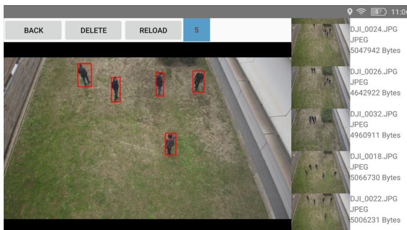
**Figure 10.** Person counting using *POLOtin* works well for low-altitude and separated targets.
