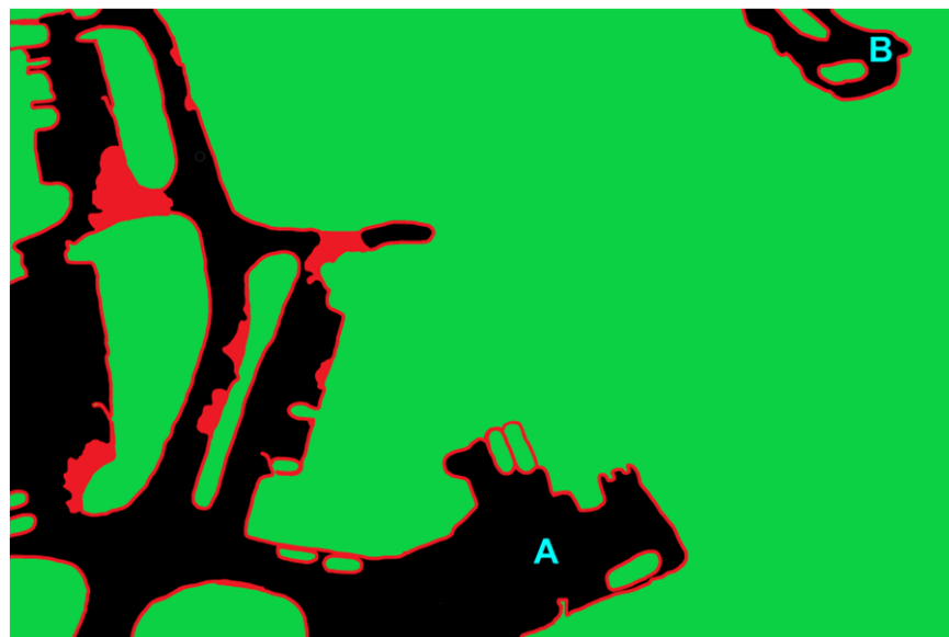
Figure 5. A sample case of image mask depicting multiple road segments that are not connected.
