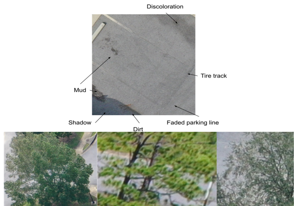
Figure 2. Top row: example of various effects on the road surface. Bottom row: examples of trees blocking view of the road in aerial footage.
