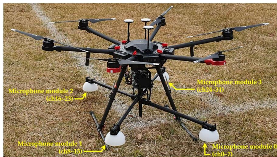
Figure 6. Microphone array system mounted on the drone.
