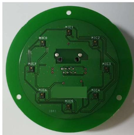
Figure 5. Microphone module consisting of 8 microphones.
