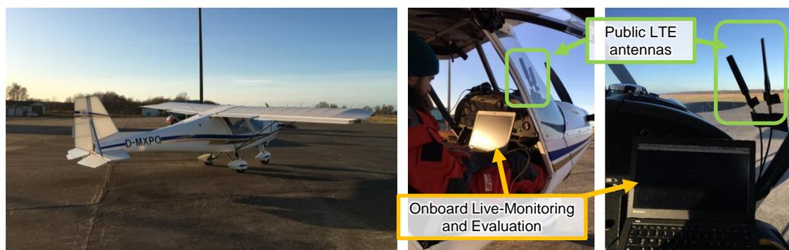
**Figure 6.** In order to evaluate maximum performance without interfering video stream and telemetry and control data flows a manned flight was conducted. The illustration shows the used ultra-lightweight aircraft and antenna position of Peenemünde flight experiment [4].
