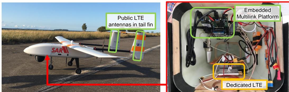
Figure 3. Illustration of the LARUS Unmanned Aerial Vehicle (UAV) showing the location of the communication hardware in front and tail fin. The UAV has a fixed wingspan for 3.6 m and a total weight of 26 kg. With its combustion, engine it is able to fly for multiple hours. All experiments except flight [4] were performed with the pictured LARUS UAV. Images: © 2020 LARUS project [1].
