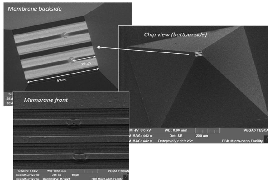
Figure 2. SEM image of the fabricated membrane with a bridge valve.
