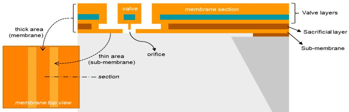
Figure 1. Membrane and bridge valve section.
