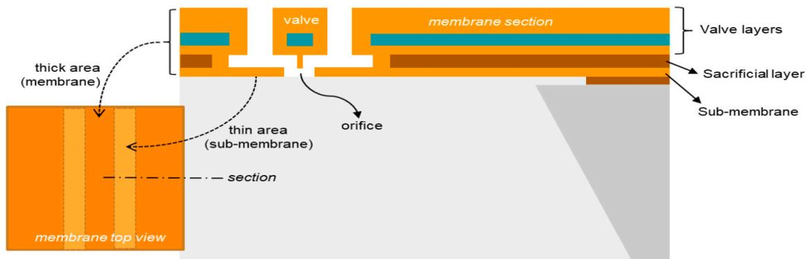
Figure 1. Membrane and bridge valve section.
