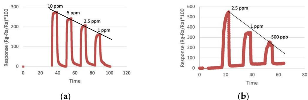
**Figure 1.** Dynamic response curves of sensors  $S_{1\text{Zac-PVA}}$ . (a) Response to NO gas in 1, 2.5, 5, and 10 ppm at 300 °C. (b) Response to NO<sub>2</sub> gas 0.5, 1, and 2.5 ppm at 300 °C.
