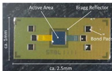
**Figure 1.** Photograph of an uncoated SMR device with the active area above a Bragg reflector [4].
