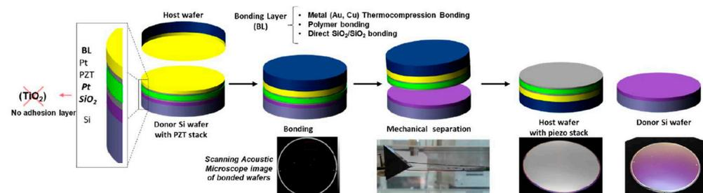
**Figure 1.** Wafer to wafer layer transfer process.
