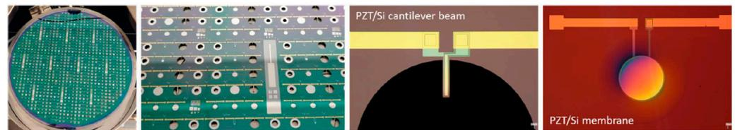
**Figure 2.** Photos of released piezoelectric MEMS structures fabricated using 200 mm Si technology.
