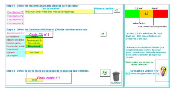
Figure 1. Result of the hand-arm OSEV tool for an angle grinder tool (meuleuse d'angle).
