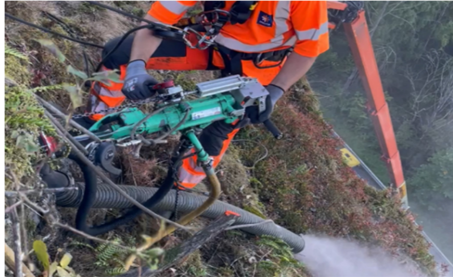
Figure 4. The prototype without ATVA being tested in the field in Norway with the dust removal device.
