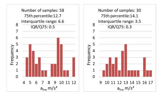
Figure 1. Examples of vibration distributions for two machine categories.
