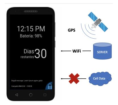
**Figure 3.** During the crowdsensing campaign, phones do not have access to a data network and run in non-interactive mode.
