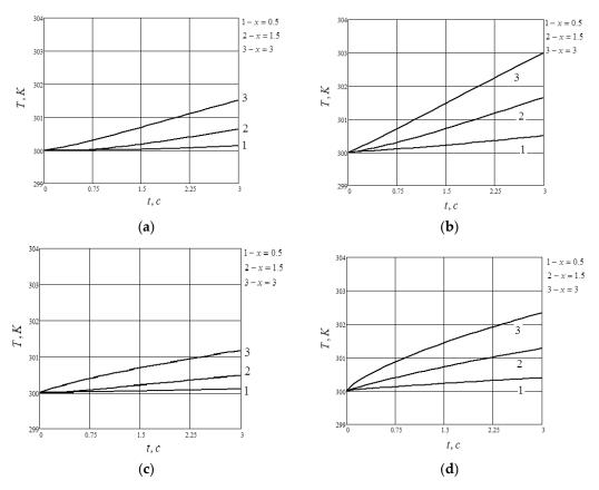
**Figure 2.** Temperature dependences on time in a semi-infinite body for: (a)  $\alpha = 1$ ,  $\beta = 2$ ; (b)  $\alpha = 1$ ,  $\beta = 1.7$ ; (c)  $\alpha = 0.7$ ,  $\beta = 2$ ; (d)  $\alpha = 0.7$ ,  $\beta = 1.7$ . For all cases:  $q_c = 1.8 \frac{\text{W}}{\text{m}^2}$ ,  $\lambda = 2.5 \frac{\text{W}}{\text{m} \cdot \text{K}}$ ,  $T_0 = 300 \text{ K}$ .
