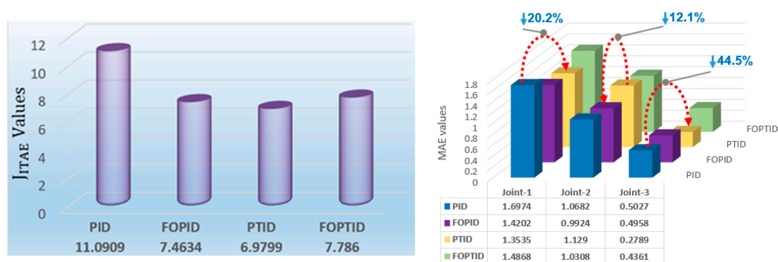
Figure 16. Comparison diagram of tracking error evaluation indicators based on J_{ITAE} and MAE values for the presented controllers.
