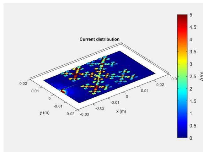
**Figure 8.** Fractal island normal antenna at 191 GHz.
