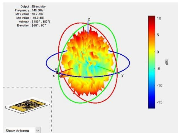
**Figure 12.** Minkowski fractal antenna pattern radiation.
