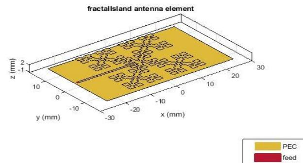
**Figure 3.** Fractal island antenna element (for third iteration).
