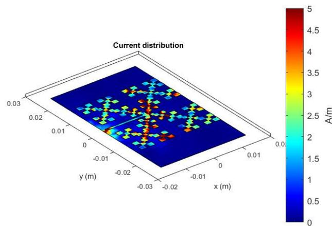
**Figure 7.** Current distribution of fractal island antenna (lateral alimentation).
