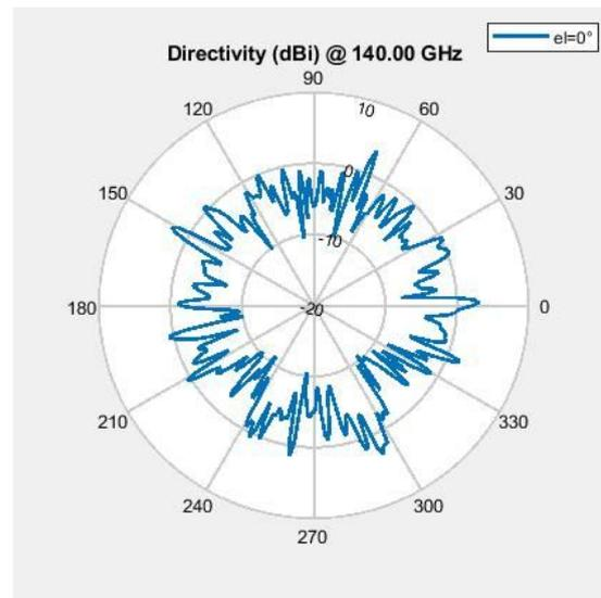
Figure 10. Azimuth pattern of Minkowski fractal antenna.
