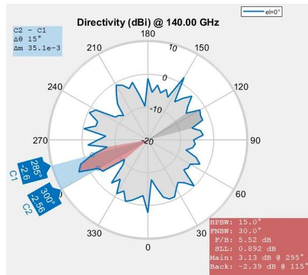
Figure 23. Azimuth pattern (directivity) of Minkowski fractal antenna.
