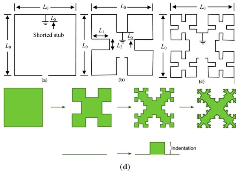
**Figure 1.** A drawing with the four iterations made (a–d), starting from the Minkowski initiator. (a) the initial start (square ring); (b) the 1st iteration; (c) the 2nd iteration; (d) the initial start (square ring) plus the first three iterations.
