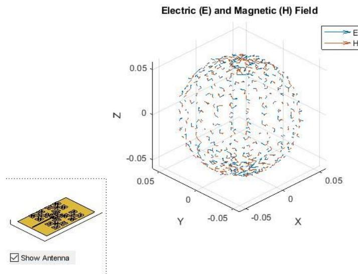
Figure 11. Electric and Magnetic Fields 3D Distribution.
