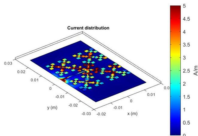
**Figure 9.** Fractal island lateral antenna at 182 GHz.
