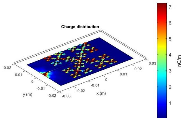
**Figure 4.** Charge distribution of fractal island antenna.
