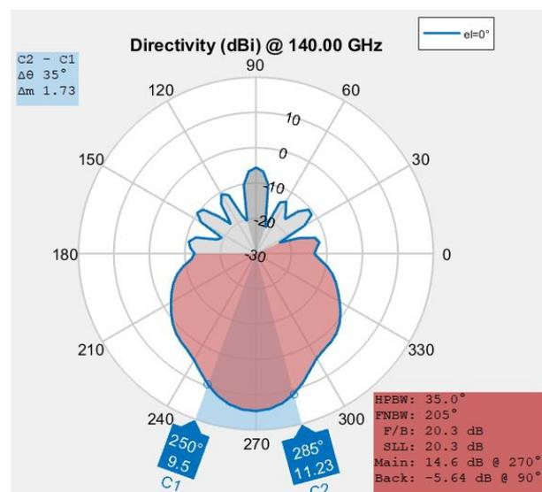
Figure 24. Azimuth pattern (directivity) of Horn antenna.
