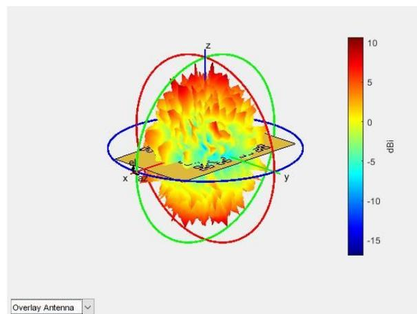
**Figure 13.** Fractal antenna pattern radiation overlay.
