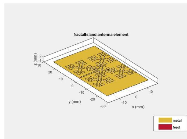
**Figure 6.** Fractal island antenna element (for fourth iteration).
