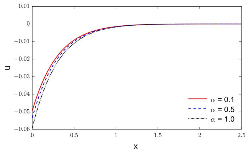
**Figure 5.** The impact of fractional parameter in the displacement variations along the distance  $x$  when  $\beta = 0.3$  and  $\tau_0 = 0.05$ .
