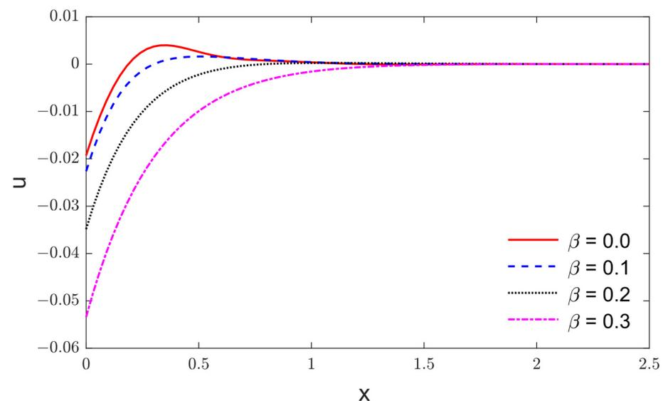
**Figure 2.** The impact of nonlocal parameter in the displacement variations along the distance  $x$  when  $\alpha = 0.3$  and  $\tau_0 = 0.05$ .
