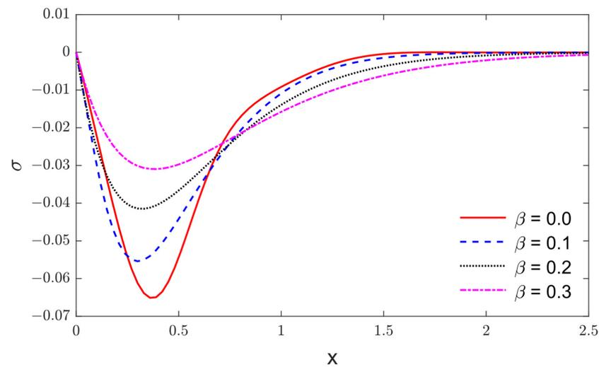
**Figure 3.** The impact of nonlocal parameter in the stress variations along the distance  $x$  when  $\alpha = 0.3$  and  $\tau_0 = 0.05$ .
