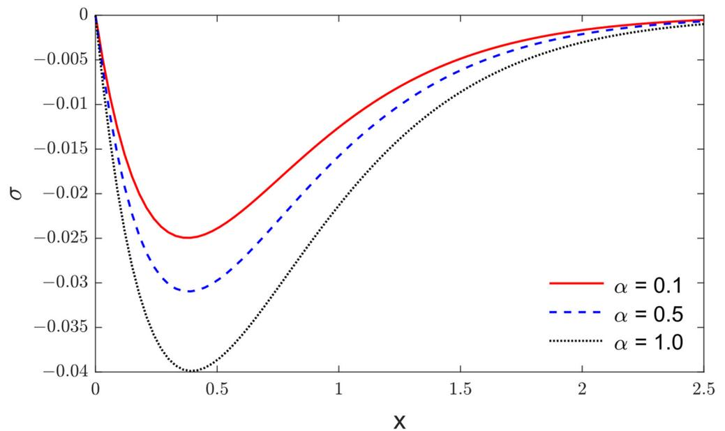
**Figure 6.** The impact of fractional parameter in the stress variations along the distance  $x$  when  $\beta = 0.3$  and  $\tau_0 = 0.05$ .
