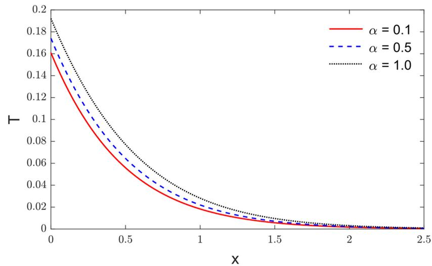
**Figure 4.** The impact of fractional parameter in the temperature variations along the distance  $x$  when  $\beta = 0.3$  and  $\tau_0 = 0.05$ .
