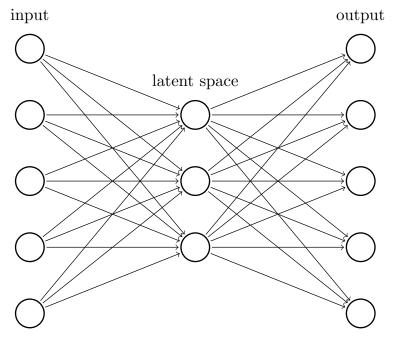
Figure 6. Schematic representation of the vanilla autoencoder used in this study.
