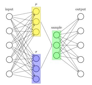
Figure 7. Schematic representation of the variational autoencoder used in this study.
