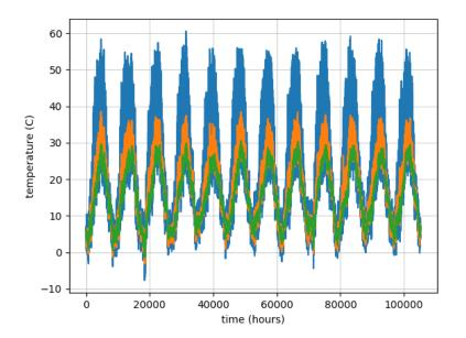
**Figure 12.** Temperature data as registered by sensors.  $T_1$  is indicated in blue,  $T_2$  is indicated in green, and  $T_3$  is indicated in orange.
