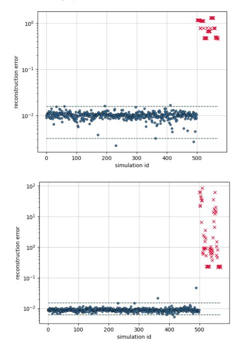
**Figure 10.** The reconstruction error for training and damaged test sets as indicated in the text for AE (**top**) and VAE (**bottom**) for the case study of the railway bridge model.
