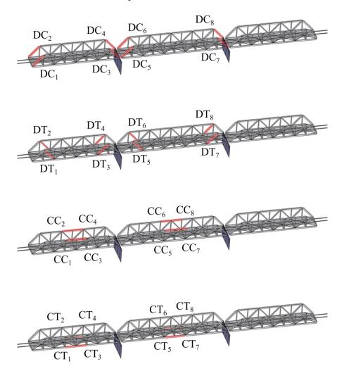
**Figure 2.** Locations of the 32 elements whose elastic modulus the user can reduce. Legend: DC, diagonal in compression; DT, diagonal in tension; CC, chord in compression; CT, chord in tension.
