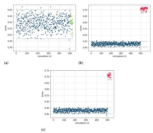
**Figure 16.** The scores, as defined in the text, corresponding to the training and the test sets for the IF. Blue points represent training set scores, green points are scores that fall within the confidence region, and red crosses are anomalies. The same three scenarios investigated using AEs are represented: no damage at all (**a**), constantly decreased elastic modulus of  $DC_1$  (**b**), and damage at 2% for each of the 32 considered beam elements (**c**).
