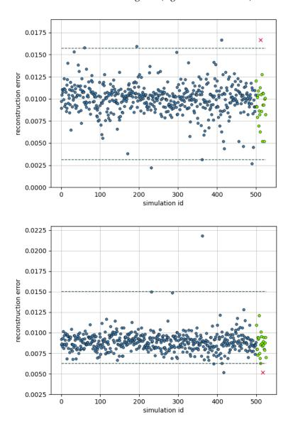
**Figure 9.** The reconstruction error for training and non-damaged test sets for AE (**top**) and VAE (**bottom**) for the case study of the railway bridge model.
