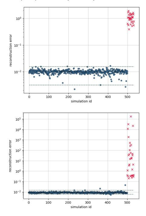
**Figure 11.** The reconstruction error for training and the second damaged test sets as indicated in the text for AE (**top**) and VAE (**bottom**) for the case study of the railway bridge model.
