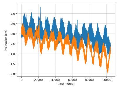
**Figure 13.** Inclinations as registered by sensors.  $I_x$  is indicated in blue, while  $I_y$  is indicated in orange.
