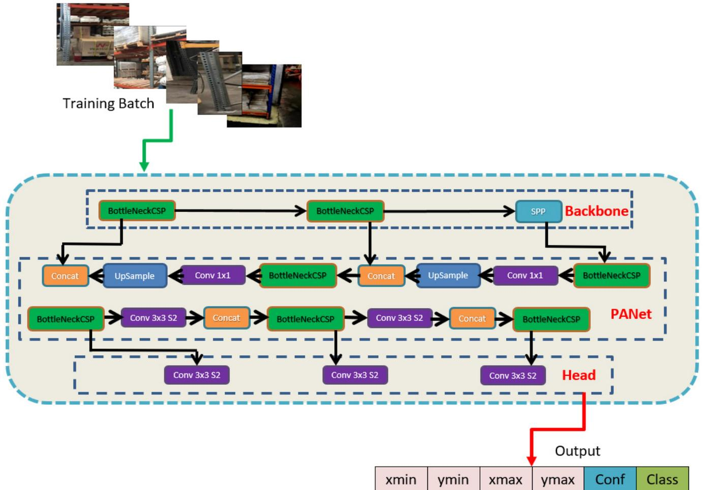
Figure 3. YOLO-v5 internal architecture.
