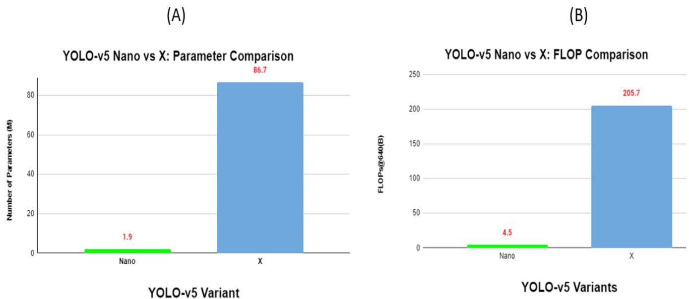
**Figure 5.** YOLO-v5 computational analysis. (A) Parameter; (B) FLOP Comparison.
