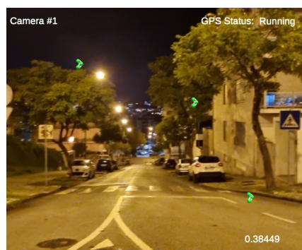
Figure 1. An example of situated visualization (SV), a context-driven visualization technique, displaying the pollution concentration related to a user's GPS coordinates on a particular street using digital augmentations based on representations of the polluting molecules.
