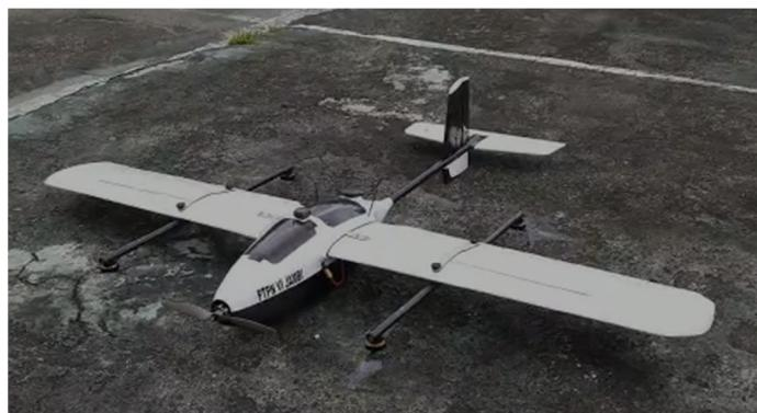
**Figure 3.** Fixed Wing VTOL drone.
