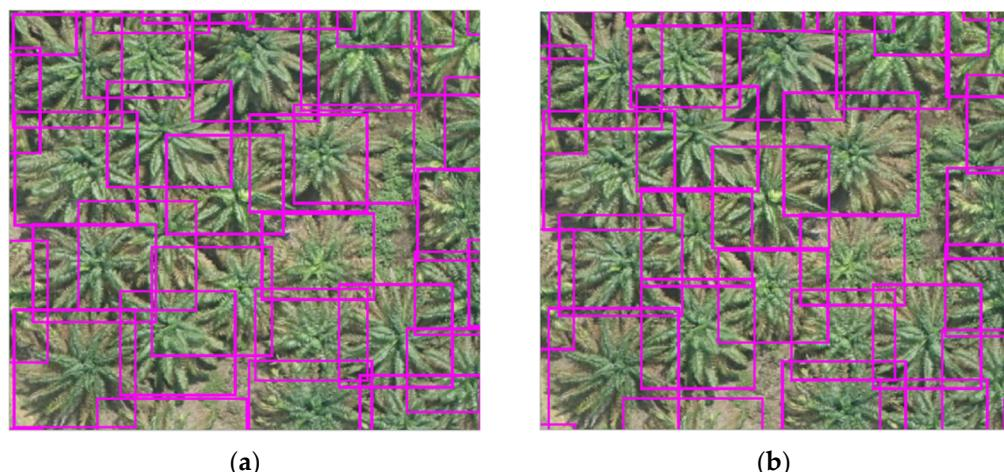
**Figure 13.** Comparison of the bounding box location to the detected object of the YOLOv3 detection results: (a) Poor accuracy on the network input size  $416 \times 416$ ; (b) Good accuracy on the network input size  $1024 \times 1024$ .
